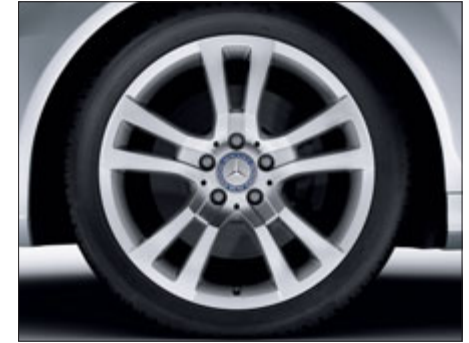
5-twin-spoke light-alloy wheels with 225/40 R 18 front tyres and 255/35 R 18 rear tyres (optional, Code R70, not in conjunction with AMG Sports package and C 63 AMG)
