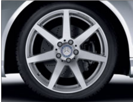
7-spoke AMG light-alloy wheels with 225/40 R 18 front tyres and 255/35 R 18 rear tyres, with high-shine finish (optional, not for C 63 AMG, Code 782)
