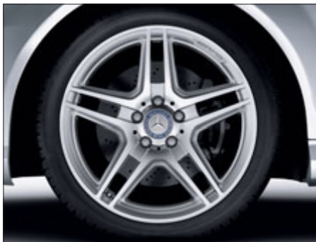
5-twin-spoke AMG light-alloy wheels with 225/40 R 18 front tyres and 255/35 R 18 rear tyres, with high-shine finish (optional, not for C 63 AMG, Code 786)
