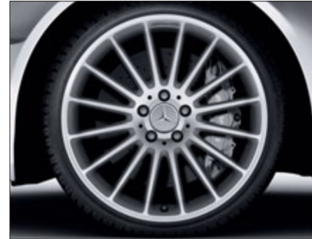
Multi-spoke AMG light-alloy wheels with 235/35 R 19 front tyres and 255/30 R 19 rear tyres, painted in titanium grey with high-shine finish (optional for C 63 AMG, Code 788)
