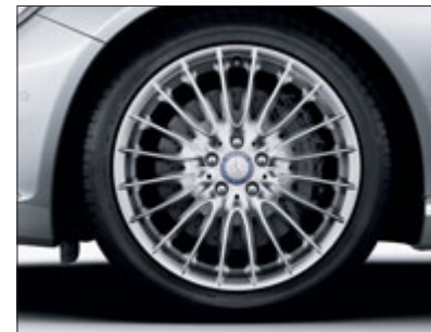
Multi-spoke light-alloy wheels with 255/40 R 19 front and 275/40 R 19 rear tyres, 255/40 R 19 tyres all round on 4MATIC models (optional)
