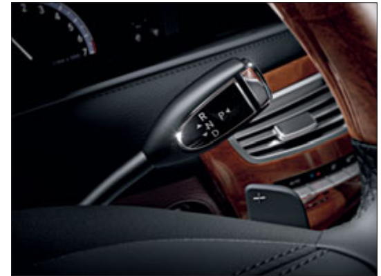
Fingertip transmission control with the DIRECT SELECT lever on the steering wheel
