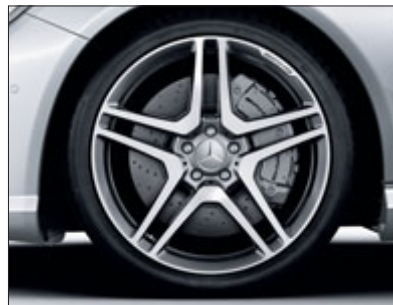
Twin-spoke AMG forged wheels with 255/35 R 20 front and 275/35 R 20 rear tyres, titanium grey, polished finish (standard for CL 65 AMG, option for CL 63 AMG)
