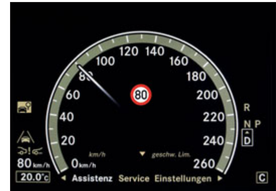
Speed Limit Assist display in the instrument cluster
