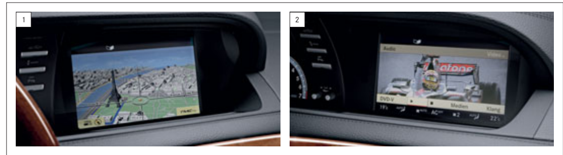
SPLITVIEW displays two different images at the same time – for the driver (1) and front passenger (2) – on a single screen
