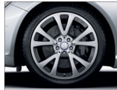
5-Y-spoke light-alloy wheels for 255/40 R 19 front and 275/40 R 19 rear tyres, 255/40 R 19 tyres all round on 4MATIC models, titanium silver, high-shine finish (optional)
