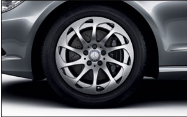
10-spoke light-alloy wheels with 245/45 R 17 tyres (standard for CLS 250 CDI BlueEFFICIENCY, Code R25)
