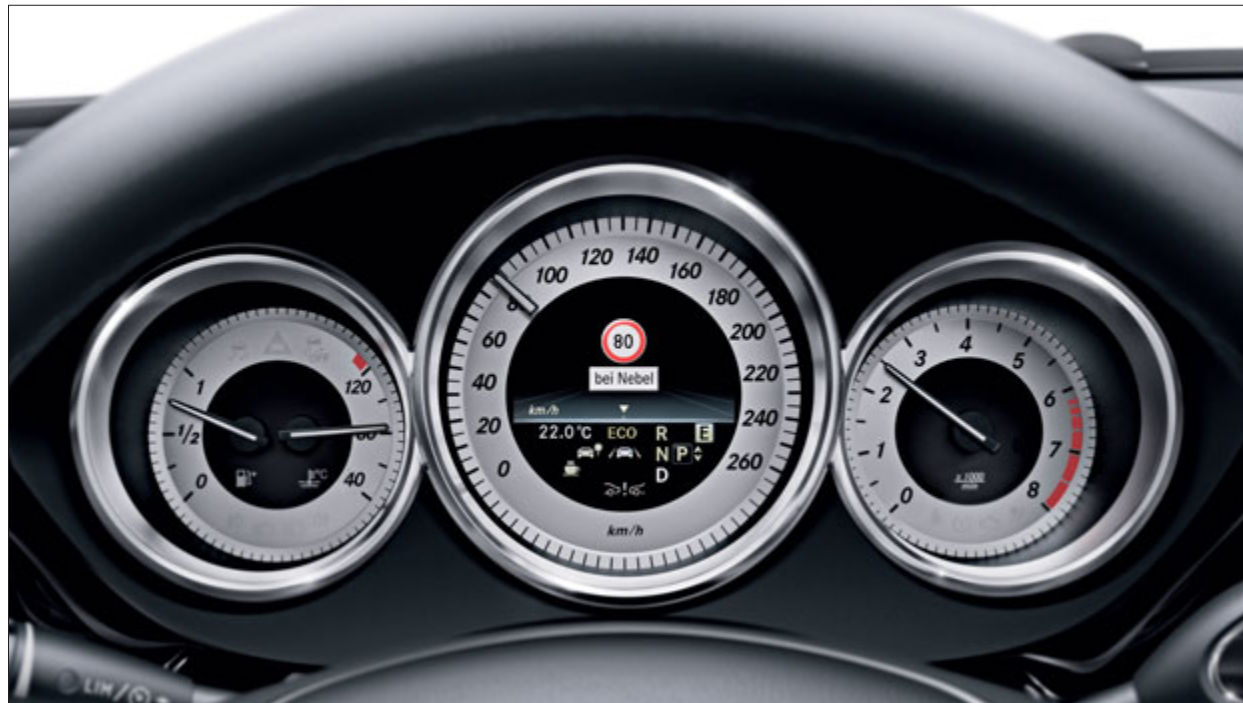
Speed Limit Assist even indicates temporary speed limits
