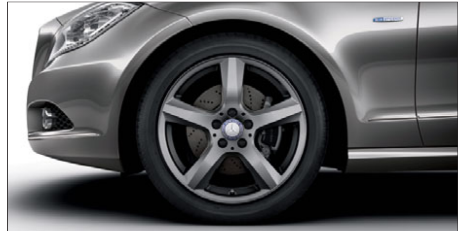
5-spoke light-alloy wheels with mixed-size tyres – front 255/40 R 18 and rear 285/35 R 18 – in anthracite
