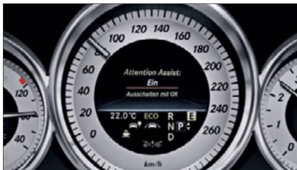
If signs of increased driver inattention or drowsiness are detected, ATTENTION ASSIST advises taking a break
