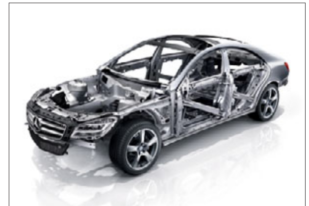
The energy-absorbing crumple zones in the front and rear sections, an extremely robust safety passenger cell, and the doors with special reinforcing elements form an effective defensive barrier in an emergency
