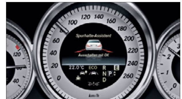
Lane Keeping Assist and Blind Spot Assist can warn the driver in potentially dangerous situations
