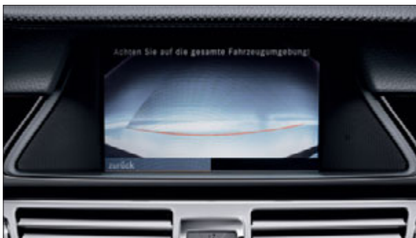
During parking, the COMAND APS central display shows the area behind the car
