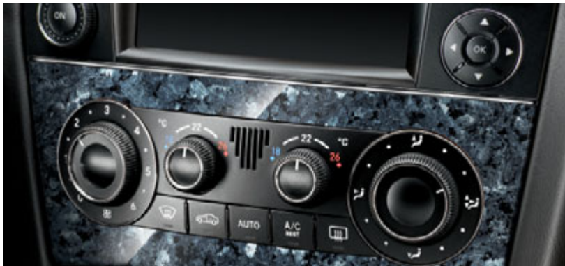
Control panel for air conditioning
