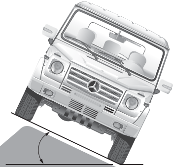
Directionally stable on lateral slopes up to 54%
