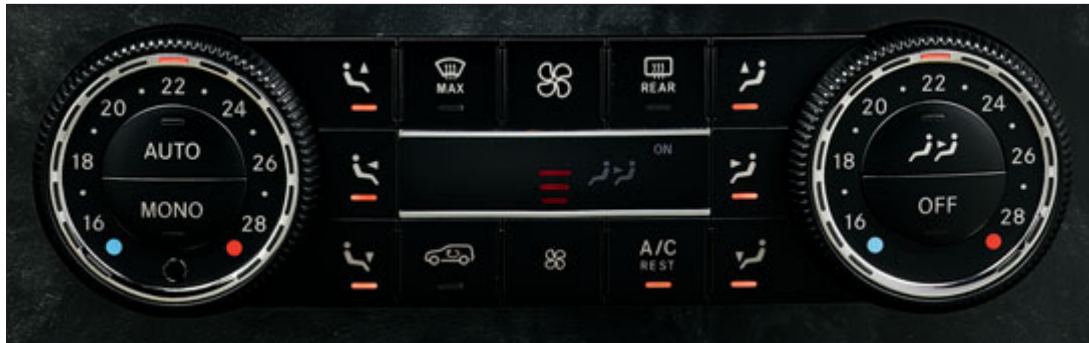
The controls for the THERMOTRONIC luxury automatic climate control system are ergonomic and intuitive
