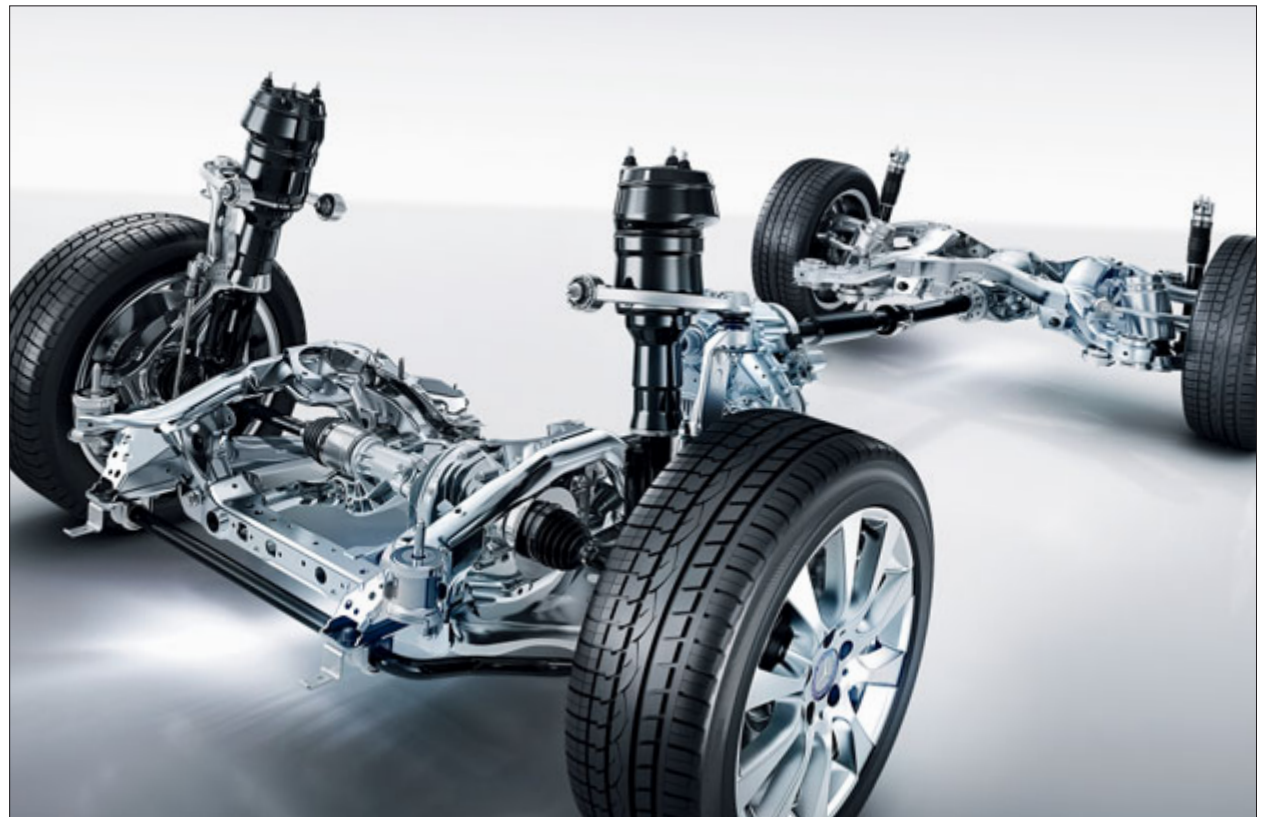
The standard suspension with selective damping system adjusts to the current driving situation and road condition quickly and precisely
