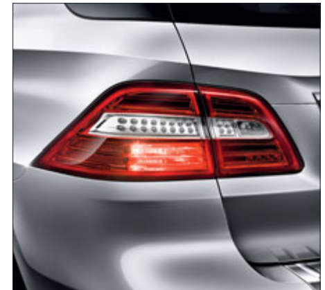
Tail lights featuring LED fibre-optic technology
