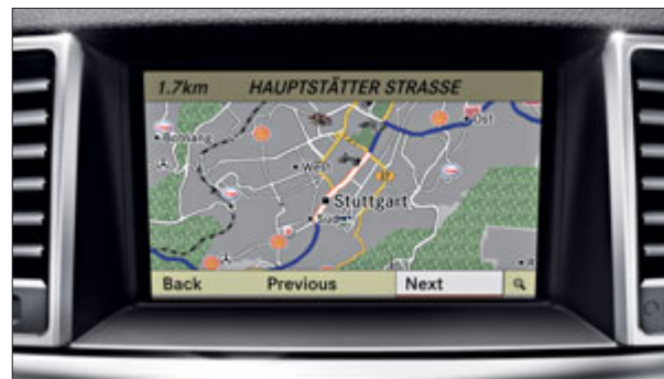
The multimedia system with HDD navigation has a high-resolution colour display with a 17.8-cm screen diagonal
