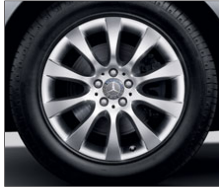
10-spoke light-alloy wheels with 255/55 R 18 tyres (standard for ML 350 4MATIC BlueEFFICIENCY, optional for diesel models, Code R41)
