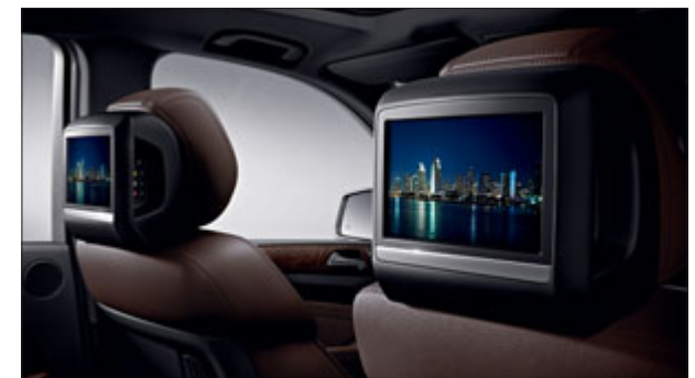
The two displays for the Rear Seat Entertainment System are mounted on the front-seat head restraints
