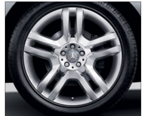
5-twin-spoke light-alloy wheels with 265/45 R 20 tyres (optional, not for ML 63 AMG, Code R33)
