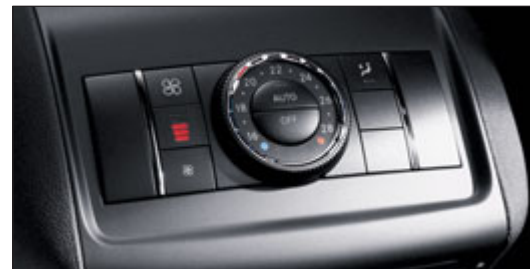
The desired temperatures and airflow can be set precisely using the control panel in the rear
