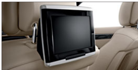
The two displays for the Rear Seat Entertainment System are mounted on the front-seat head restraints
