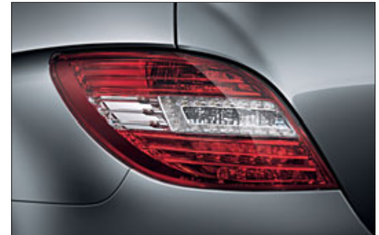
Tail light featuring LED and fibre-optic cable technology
