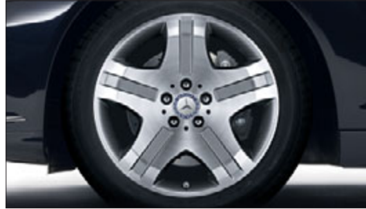
5-spoke light-alloy wheel with 255/45 R 18 front and 275/45 R 18 rear tyres (standard for V12 engine)
