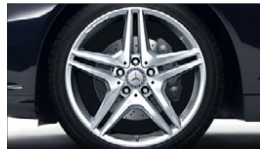
AMG 5-twin-spoke light-alloy wheel with 255/35 R 20 front and 275/35 R 20 rear tyres (optional extra)
