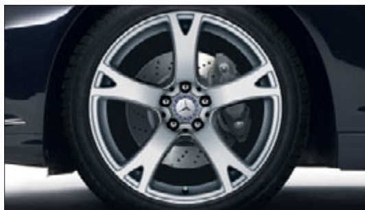
5-spoke light-alloy wheel with 255/40 R 19 front and 275/40 R 19 rear tyres (optional extra)
