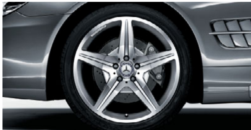
5-spoke AMG light-alloy wheels, with high-shine finish, with 255/35 R 19 front tyres and 285/30 R 19 rear tyres
