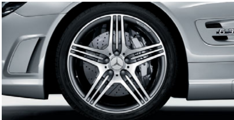
Triple-spoke AMG light-alloy wheels with high-shine, titanium-grey painted finish, with 255/35 R 19 front tyres and 285/30 R 19 rear tyres (standard for SL 63 AMG)
