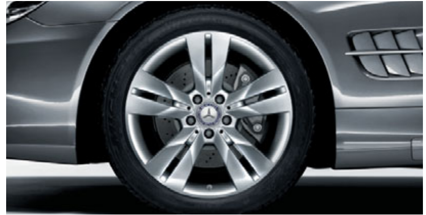
5-twin-spoke light-alloy wheels, with high-shine finish, with 255/40 R 18 front tyres and 285/35 R 18 rear tyres (optional extra)
