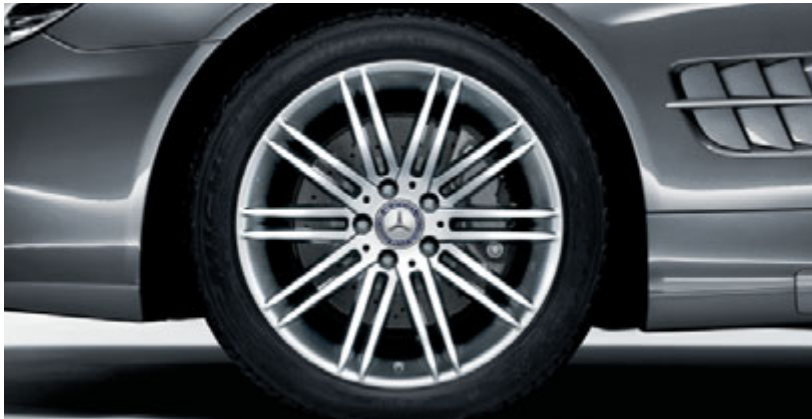
V12-design light-alloy wheels with 255/40 R 18 front tyres and 285/35 R 18 rear tyres (standard for SL 600)
