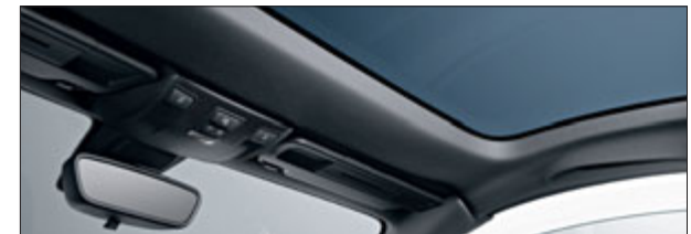
MAGIC SKY CONTROL enables adjustment of the optional panoramic vario-roof's transparency
