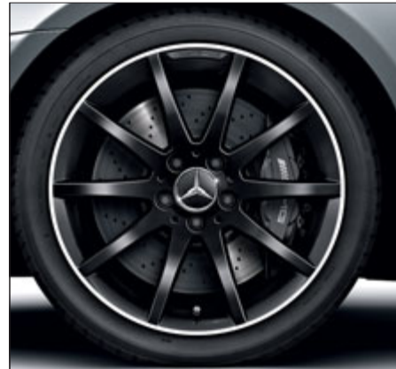
Multi-spoke AMG light-alloy wheels, painted black, rim flange with high-sheen finish, with 235/40 R 18 front and 255/35 R 18 rear tyres (Code 760)
