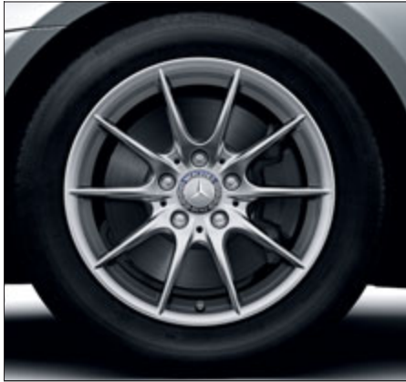
10-spoke light-alloy wheels with 205/55 R 16 tyres (standard for SLK 200 BlueEFFICIENCY, Code 39R)
