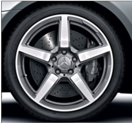
5-spoke AMG light-alloy wheels, painted titanium grey with a high-sheen finish, with 235/40 R 18 front and 255/35 R 18 rear tyres (Code 790)
