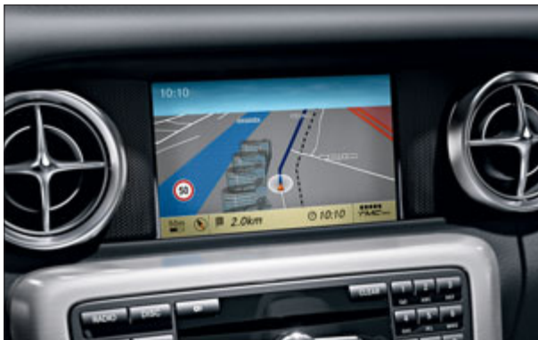
The information from the Speed Limit Assist is shown on both the instrument cluster and the COMAND Online central display
