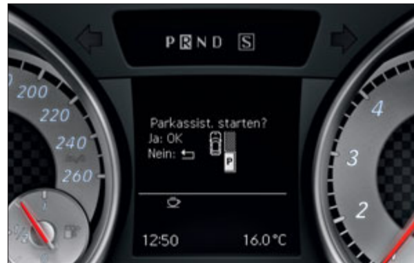
Parking Guidance indicates suitable parking spaces to the driver and provides parking directions
