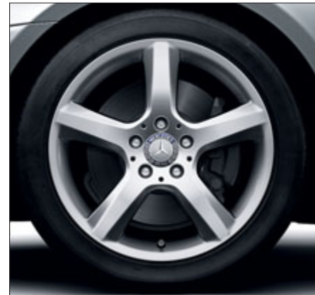
5-spoke light-alloy wheels with 225/45 R 17 front and 245/40 R 17 rear tyres (standard for SLK 250 BlueEFFICIENCY, Code 37R)
