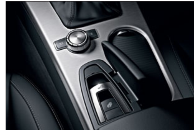
Roof controls and Controller
