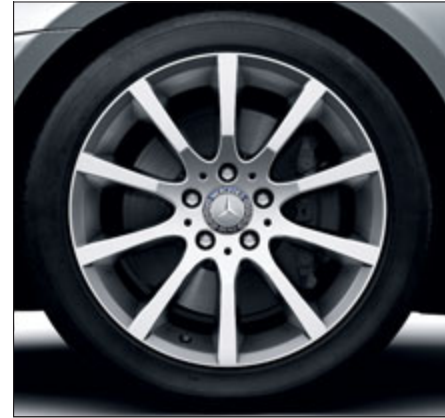
10-spoke light-alloy wheels with 225/45 R 17 front and 245/40 R 17 rear tyres (standard for SLK 350 BlueEFFICIENCY, Code R35)
