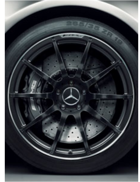
Optional extra. 10-spoke AMG forged wheels, painted matt black, rim flange with a high-sheen finish
