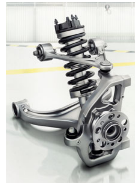
AMG RIDE CONTROL suspension, Adaptive Damping System with three driving modes
