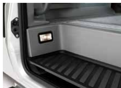
Illuminated step exit. Helps passengers exit safely even at night.
