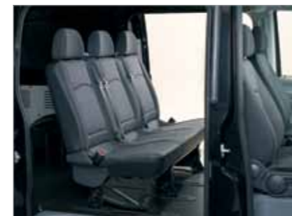
Second row of seats can be removed to create more cargo room
