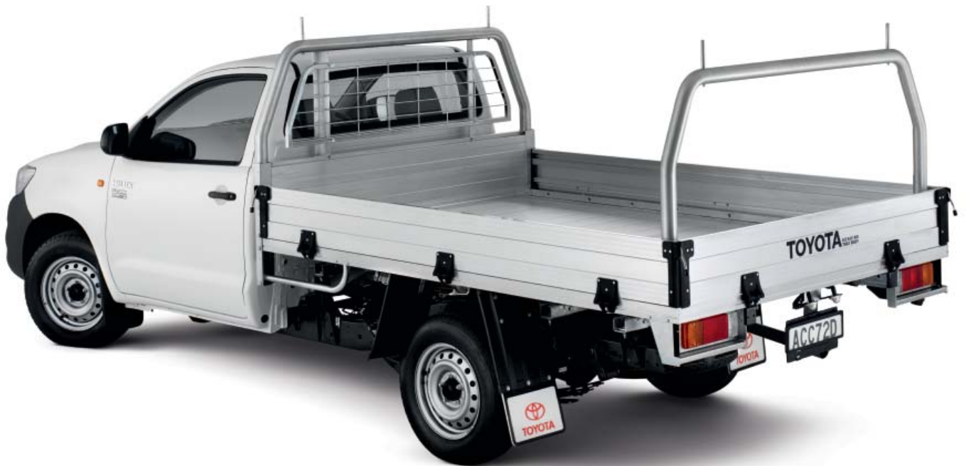
4x2 WorkMate Single-Cab Cab-Chassis featuring Heavy Duty Alloy Tray with optional headboard shown.
