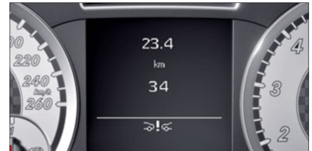
The COLLISION PREVENTION ASSIST can recognise a safety margin that is too short and warn the driver
