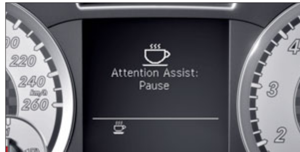
The ATTENTION ASSIST recommends taking a break if it detects signs of driver drowsiness or inattention
