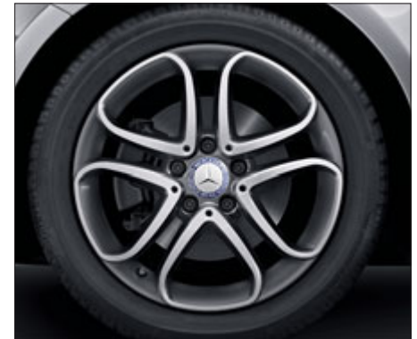
5-twin-spoke light-alloy wheel, painted himalayas grey, with a high-sheen finish and 225/45 R 17 tyres (option, not in conjunction with AMG Sport, Code R48)
