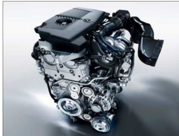
The newly developed 4-cylinder A 180 BlueEFFICIENCY petrol engine boasts direct injection via piezo injectors and a turbocharger
