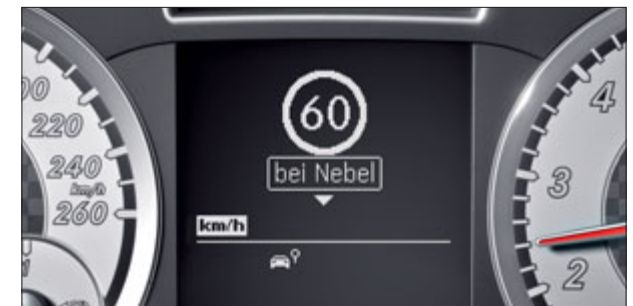
The information from Speed Limit Assist is shown both in the instrument cluster and in the COMAND Online central display
