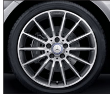
Multi-spoke AMG light-alloy wheel, painted titanium grey, with a high-sheen finish and 225/40 R 18 tyres (standard in conjunction with AMG Sport, Code 791)
