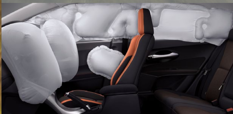
Driver and front passenger SRS airbags, front seat side airbags, full length side curtain shield airbags and driver's knee airbag. Levin model shown.
