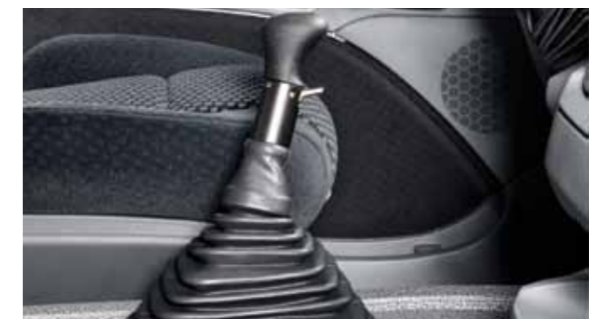
The hydraulic gearshift is a manual gearshift with hydraulic force transmission and pneumatic assistance. Only available with selected transmissions.
