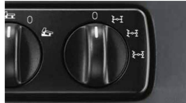
The standard-fit differential locks are operated by means of a rotary switch and according to a simple logic the differentials are locked in the following sequence: inter-axle lock, rear driven axles and finally the driven front axles.
