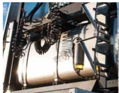
900-litre fuel tank mounted in the rear gantry is standard.
