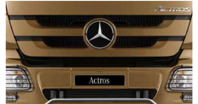
New, optimised steel protective grilles are available upon request for the headlamps and the tail lamps of the Actros. They prevent damage by stone chippings or gravel or other bulk material. This way they contribute to reducing repair costs and increasing safety.
