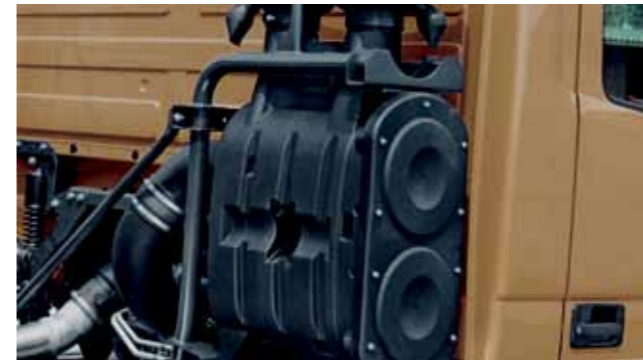
Tandem air filter system: The powerful tandem air filter system is fitted at the right, behind the cab and features an upstream cyclone unit.
