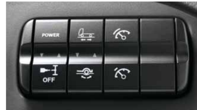
Mercedes PowerShift 2 in the Actros helps to ensure greater ride comfort, safety and economy thanks to the five specifically selectable programmes: Power Mode, Ecofuel Mode, Manoeuvring Mode, Rocking Mode and Extended Cruise Control range, where the speed range for drive and brake cruise control is wider and freely selectable. In addition, practical supplementary functions such as the ability to shift directly from 1 to R, high-ratio reverse gears and a kick-down function made for improved vehicle handling and better driver comfort. The instrument cluster shows the operating status and the currently active Mercedes PowerShift programme in the matrix display.
