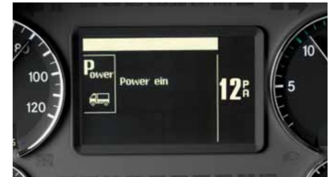
Mercedes PowerShift 2 in the Actros helps to ensure greater ride comfort, safety and economy thanks to the five specifically selectable programmes: Power Mode, Ecofuel Mode, Manoeuvring Mode, Rocking Mode and Extended Cruise Control range, where the speed range for drive and brake cruise control is wider and freely selectable. In addition, practical supplementary functions such as the ability to shift directly from 1 to R, high-ratio reverse gears and a kick-down function made for improved vehicle handling and better driver comfort. The instrument cluster shows the operating status and the currently active Mercedes PowerShift programme in the matrix display.
