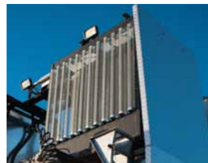
The rear gantry houses the auxiliary cooling equipment to ensure vehicle performance in the most extreme conditions.
