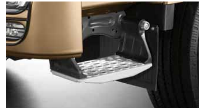
The hinged steps are specially designed for vehicle operation on construction sites and on difficult terrain. The steps are attached at the mounting points on the vehicle. They are mounted using rubber elements that are capable of longitudinal and transverse movement. Mounting in rubber bearings reduces damage due to transverse loads and also prevents corrosion damage.
