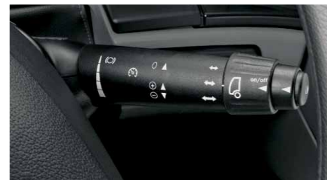
The combined drive and braking cruise control included as standard accelerates the vehicle to the set speed on uphill gradients – and if necessary it brakes the truck to the speed you have pre-set when going downhill.
