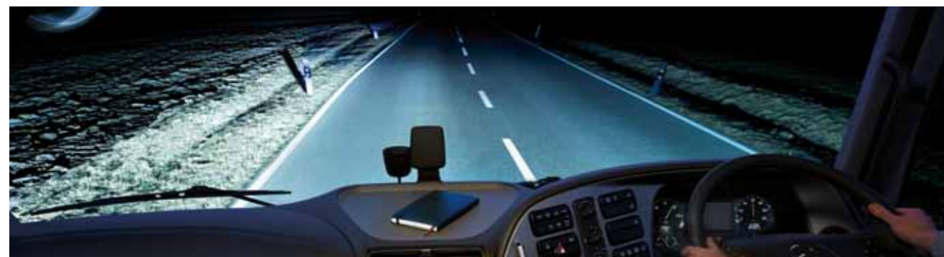
A bi-xenon version of the clear-lens Actros headlamps is also available as an option. With a range of 65m using low-beam headlamps and a range of 180m using the main beam, these headlamps provide very good visibility in the darkness, similar to daylight conditions, which in turn means better safety. Fog lamps for the front apron are also available on request.
