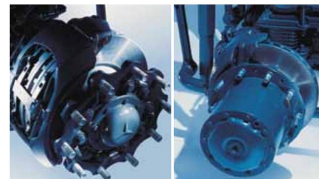
Disc brakes with EBS provide effective and efficient braking.
