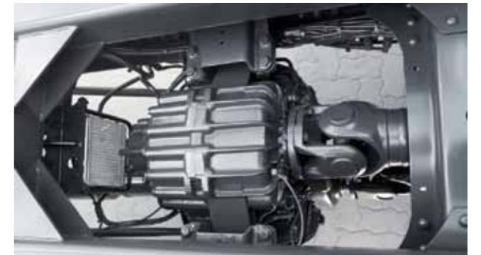
The 2-speed VG 2400 transfer case distributes the power of the drive shaft to the front and rear axle(s). Drive is permanent, i.e. the individual axles do not need to be connected or disconnected separately. The three-shaft transfer case has one-road ratio, one off-road ratio and a connectable centre differential lock.
