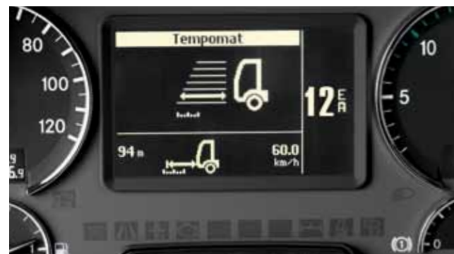
The Telligent® proximity control optionally available in conjunction with a retarder allows more relaxed and safe driving. This is because the speed and gap maintained by the Actros are automatically adjusted by the drive and braking cruise control as the traffic situation changes.
