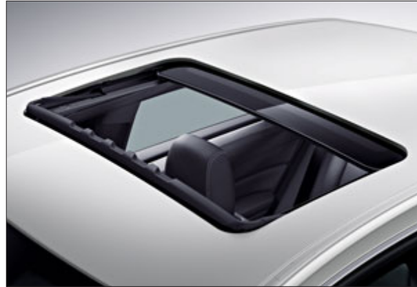
Sliding glass sunroof, electrically operated.
