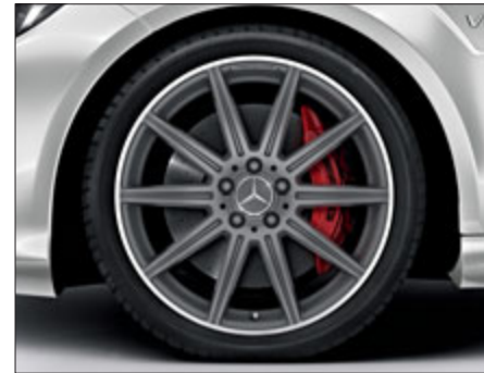
10-spoke AMG light-alloy wheels with 255/35 R 19 tyres at the front and 285/30 R 19 tyres at the rear, painted titanium grey matt, rim flange with high-sheen finish (standard only for E 63 AMG S-Model 4MATIC, Code 662).
