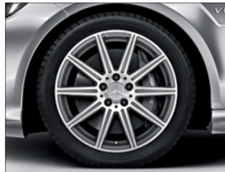
10-spoke AMG light-alloy wheels with 255/35 R 19 tyres at the front and 285/30 R 19 tyres at the rear, with high-sheen finish (Code 797 3 /796 4 ).
