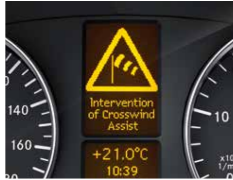
Crosswind Assist. 1 Provides for automatic intervention by the brake system in the event of strong, gusty crosswinds in order to help the vehicle stay on course. This enhances safety and provides peace of mind for the driver.
