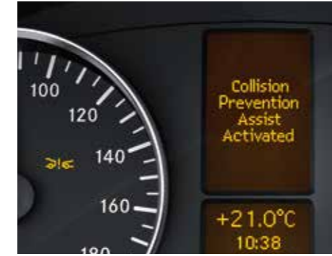
COLLISION PREVENTION ASSIST. 4 Provides visible and audible warnings if the distance to another vehicle or obstacle is insufficient and uses BAS PRO to assist the driver in the event of emergency braking.
