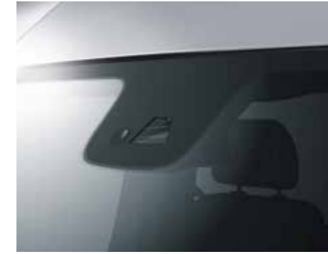
Highbeam Assist. 4 Optimum vision through automatic control of main beam activation depending on the surroundings and traffic situation.
