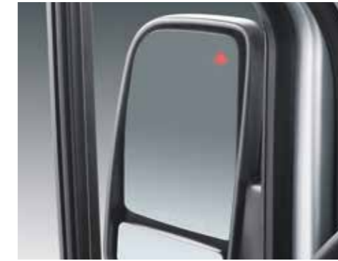
Blind Spot Assist. 4 Helps to avoid accidents by detecting vehicles in the blind spot and giving the driver visible and audible warnings.
