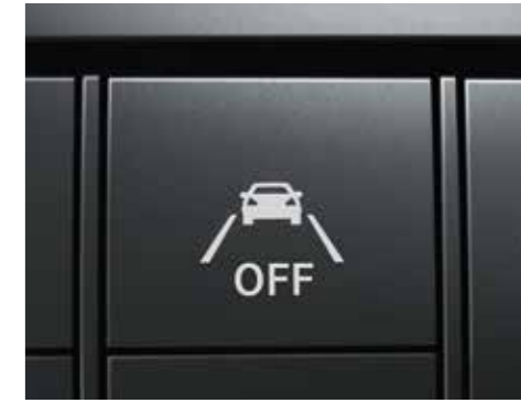
Lane Keeping Assist. 4 Lane Keeping Assist gives the driver audible and visible warnings if the vehicle leaves its lane unintentionally.
