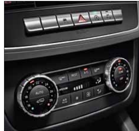
THERMATIC automatic climate control with 2 climate zones.
