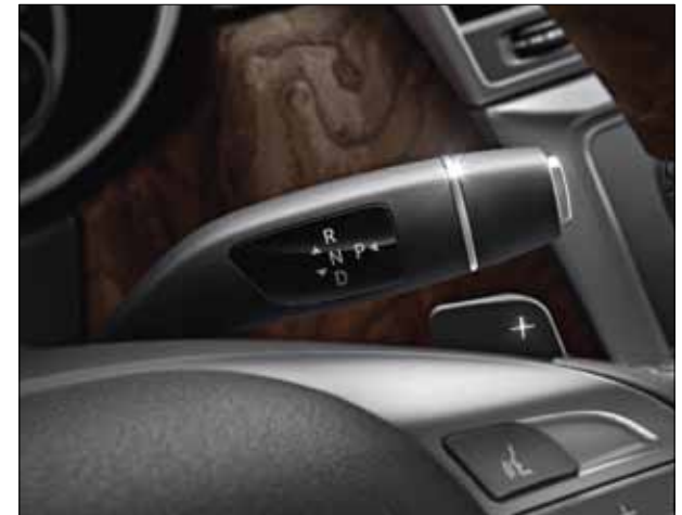
The driver can intervene manually in the gear selection using either the DIRECT SELECT lever or the shift paddles on the steering wheel.
