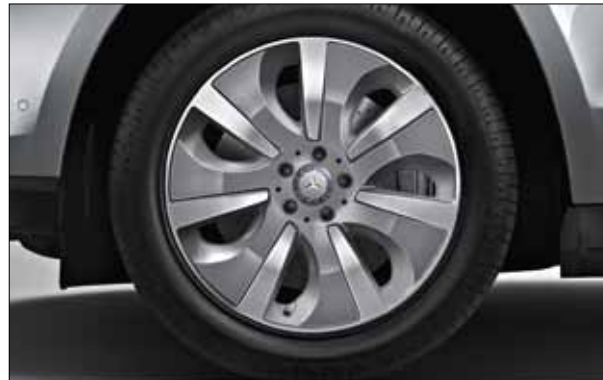
7-spoke light-alloy wheels with 275/55 R 19 tyres (optional, Code 06R).
