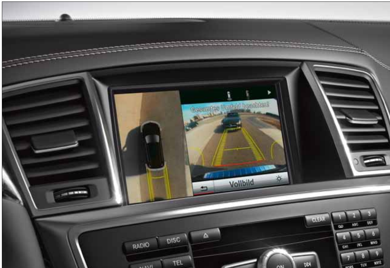
The 360° camera produces an image of the GL-Class and its immediate surroundings from a bird's-eye view.
