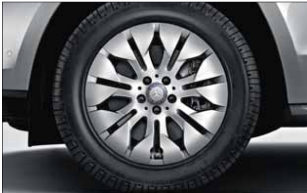
7-spoke light-alloy wheel with 265/60 R 18 tyres (optional, Code 52R).
