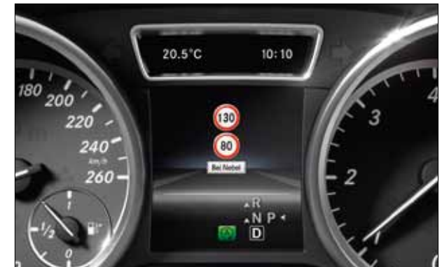
Speed Limit Assist can also display temporary speed limits in the instrument cluster.
