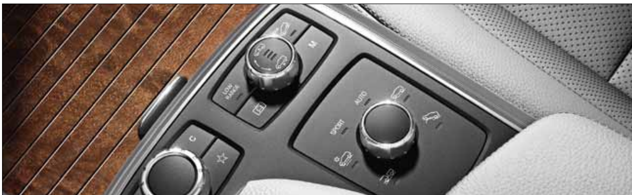
A rotary switch in the centre console is used to set the desired driving mode.
