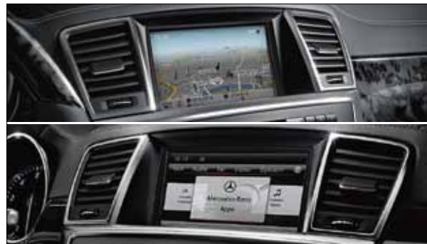
SPLITVIEW shows the driver and front passenger different content at the same time.
