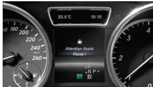
If ATTENTION ASSIST detects signs of driver drowsiness it recommends taking a break.
