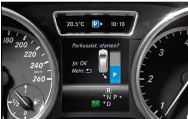
The system completes the automatic parking procedure in a maximum of five moves.
