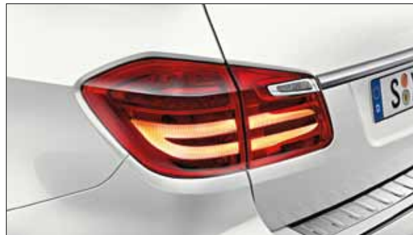
The lights in LED fibre-optic technology dominate the tail-end view of the GL-Class.
