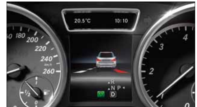
Can warn of unintended lane changes and intervene if necessary: Active Lane Keeping Assist.
