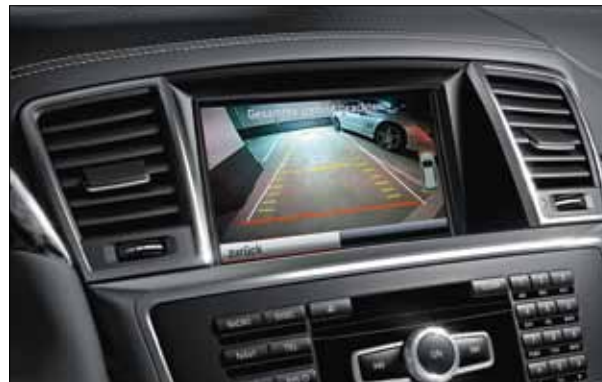
During parking, the COMAND Online central display shows the area behind the car with the reversing camera.
