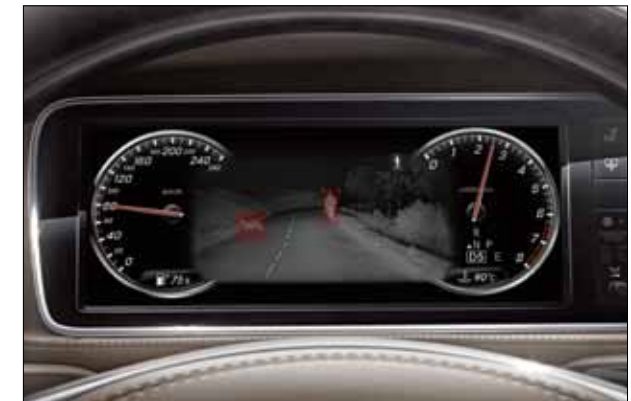
Night View Assist Plus highlights any people it has recognised and helps the driver to react more quickly to dangers at night.
