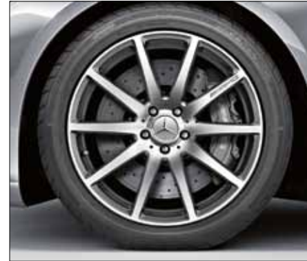
AMG 10-spoke forged wheel painted in titanium grey and polished, with 255/45 R 19 front tyre and 285/40 R 19 rear tyre (standard for S 63 and S 63 AMG 4MATIC, Code 788).
