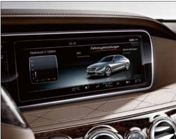
SPLITVIEW displays two different images at the same time – for the driver and front passenger – on a single screen in the centre console.
