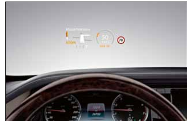
The head-up display posts information directly within the driver's field of vision.
