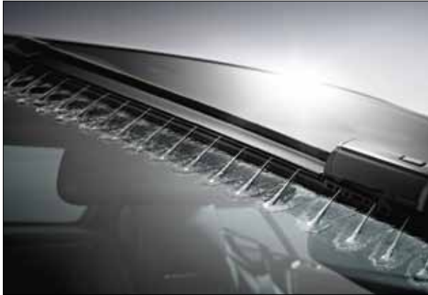
The MAGIC VISION CONTROL adaptive wiper system.
