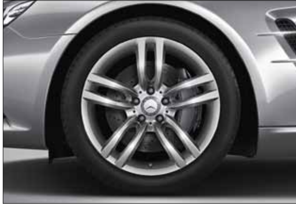
5-twin-spoke light-alloy wheels, painted vanadium silver, with 255/40 R 18 front tyres and 285/35 R 18 rear tyres (option, Code R70).
