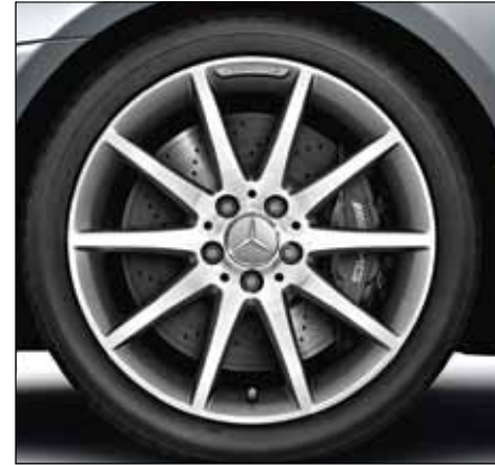
10-spoke AMG light-alloy wheels, painted titanium grey, high-sheen, with 235/40 R 18 front and 255/35 R 18 rear tyres (option, Code 796).
