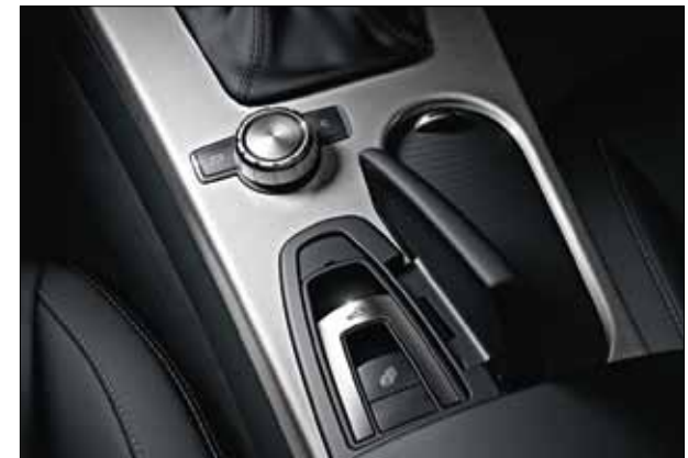
Roof control unit and Controller.
