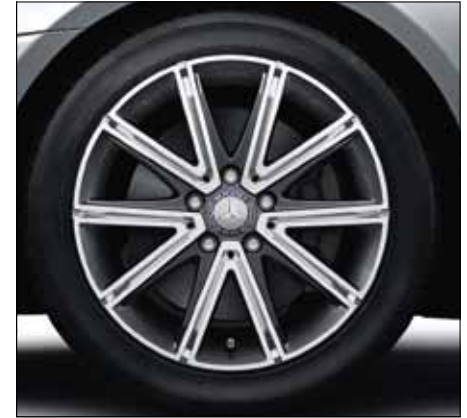
10-spoke light-alloy wheels, painted palladium silver, high-shine, with 225/45 R 17 front and 245/40 R 17 rear tyres (option, Code R93).
