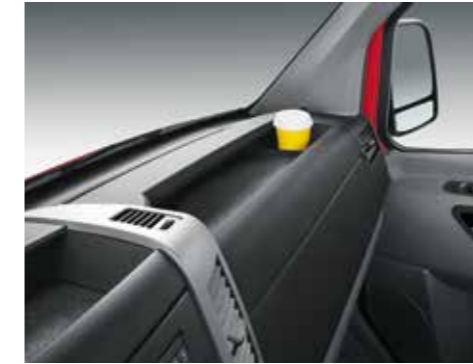
Stowage facilities in the cockpit. Generous stowage includes plenty of handy storage space (e.g. compartment above the windscreen) and several cup holders.
