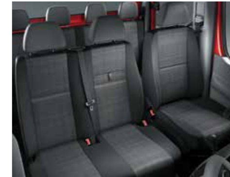
Crewcab (interior appointments). For up to 7 people, including the driver; with 4-person rear bench seat as standard, twin co-driver's seat as an option and 2-way head restraints on all seats.
