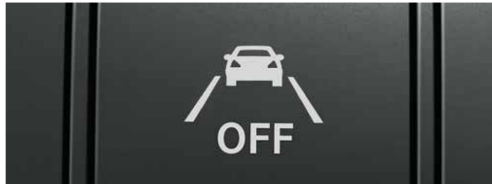
Lane Keeping Assist! Lane Keeping Assist gives the driver audible and visible warnings if the vehicle leaves its lane unintentionally.
