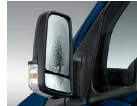
Electrically operated exterior mirrors. The rear-view mirrors on the exterior and the additional wide angle mirror are electrically adjustable and heated.
