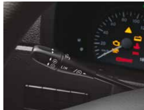
Cruise control with SPEEDTRONIC. Variable speed limiter SPEEDTRONIC assists the driver in adhering to speed limits by setting a maximum speed.
