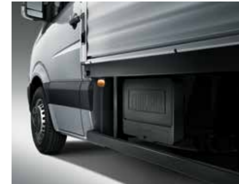
Side underride guard. The sturdy tubular steel frame protects vehicle components and reduces the risk of injury, for example, in a lateral collision. 2
