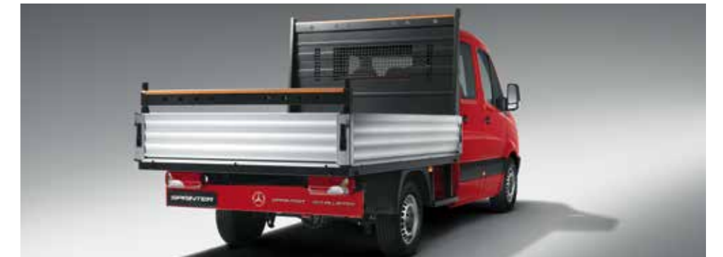
Ladder rack. Enables long objects to be secured in place. Installed behind the cab to protect it against damage.
