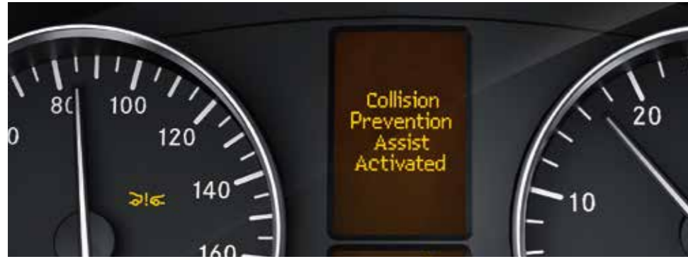
COLLISION PREVENTION ASSIST! Provides visible and audible warnings if the distance to another vehicle or obstacle is insufficient and uses BAS PRO to assist the driver in the event of emergency braking.
