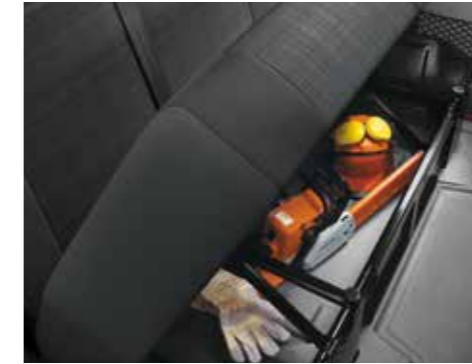
Stowage space beneath the rear bench seat (crewcab). There is a stowage compartment beneath the 4-person rear bench seat – ideal for storing long, bulky objects.
