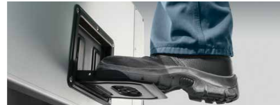
Metal step. Attached to the inner wall of the tailboard, the step makes it easier to access the platform.
