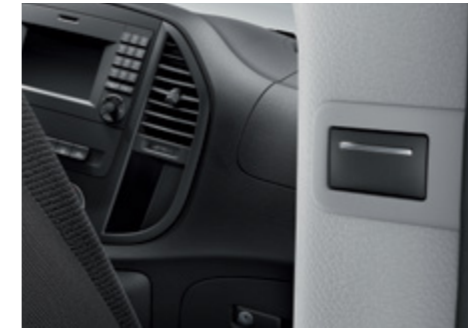
The electrically operated sliding door on the right can be opened and closed at the touch of a button.
