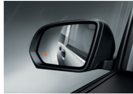
Blind Spot Assist can reduce the risk of accidents when changing lanes, for example on freeways.
