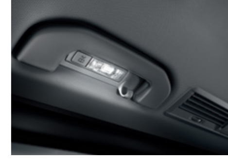
The interior and ambient illumination enhances comfort and includes a reading light in the grab handle and courtesy lights.
