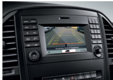
The reversing camera shows a photorealistic image of your surroundings with dynamic guide lines and an indication of the direction of travel.
