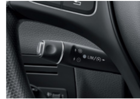
Cruise control helps to maintain a set speed, making the driver's job easier.
