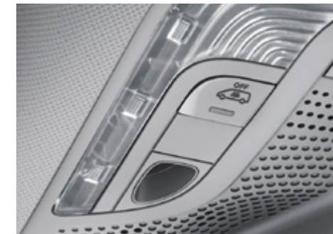
Antitheft protection package - features towaway protection, interior surveillance and alarm.
