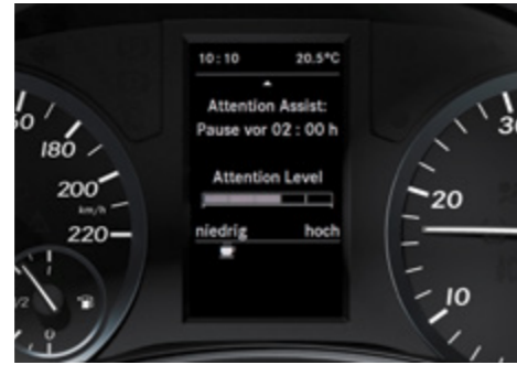
ATTENTION ASSIST can use a variety of parameters to detect signs of tiredness and alert the driver. Overseas model shown.
