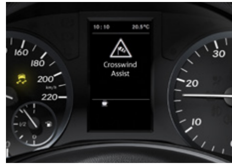
Crosswind Assist helps to reduce lateral displacement in gusty side winds.
