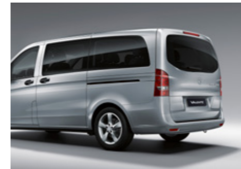
The black tinted windows in the rear provide protection from prying eyes and reduce solar heat and UV transmission in the passenger compartment.
