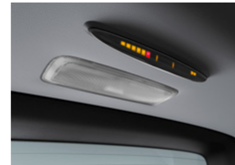
PARKTRONIC - front and rear sensor detect obstacles and provide audio and visual warnings.
