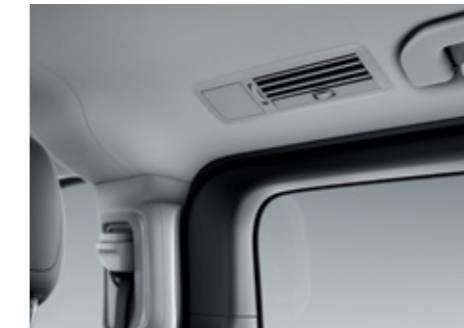
TEMPMATIC semi-automatic climate control in the rear optimises ventilation in the passenger compartment with evenly distributed warm or cool air.
