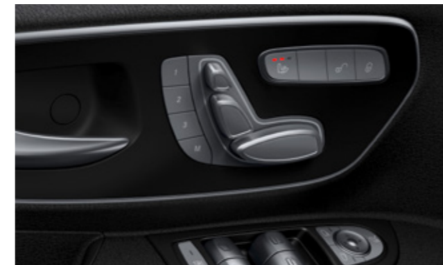
Electric seats with memory function, seat heating and the multiple award-winning PRE-SAFE® system which is able to activate precautionary occupant protection measures in critical driving situations.
