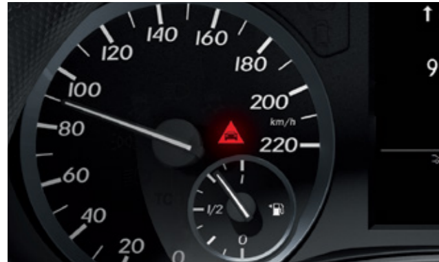
COLLISION PREVENTION ASSIST combines a distance and collision warning with Brake Assist BAS PRO.
