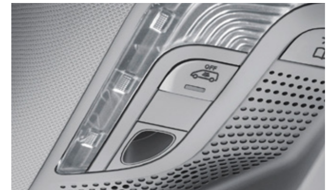
Antitheft protection package - features towaway protection, interior surveillance and alarm.
