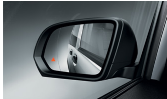
Blind Spot Assist can reduce the risk of accidents when changing lanes, for example on freeways.
