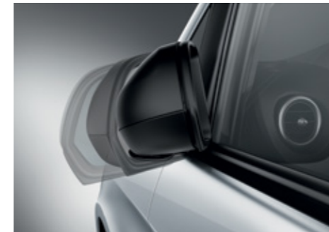
The mirror package includes automatically dimming mirrors and electrically folding exterior mirrors.
