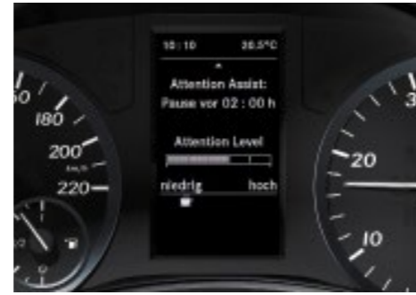
ATTENTION ASSIST can use a variety of parameters to detect typical signs of tiredness and alert the driver. *Overseas model shown.
