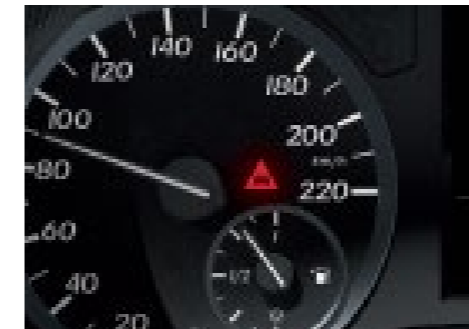
COLLISION PREVENTION ASSIST combines a distance and collision warning with Brake Assist BAS PRO.
