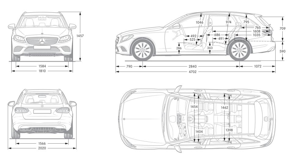
All figures in millimetres. The illustrated dimensions are mean values. They are valid for vehicles in basic specification and in unladen condition.
