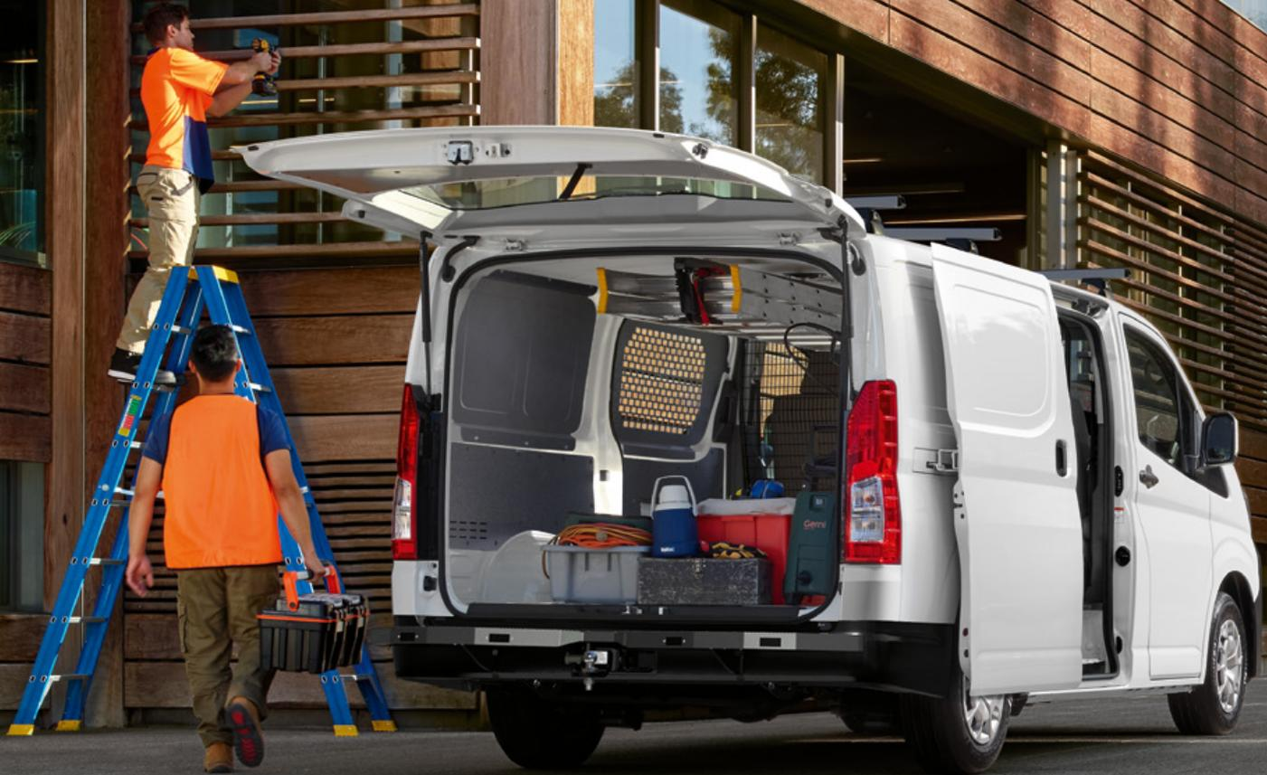
HiAce LWB Crew Van model shown accessorised with roof racks, interior wall protectors, interior ladder rack (ladder sold separately), cargo barrier, rear technician step with tow bar, tow ball and trailer wiring harness. All accessories sold separately.
