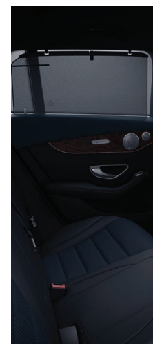
Roller sunblinds in rear side 313
