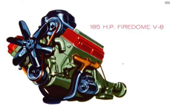
Famous for smooth, eager power and top economy (on regular gas), the Firedome V-8 for 1955 is increased to a hefty 185 horsepower. Precision-built for quietness, greater smoothness and long life, Firedome's bore and displacement have been increased for greater power... it has larger intake and exhaust valves for better "breathing"... new 2-barrel carburetor... and an improved camshaft for smoother idle.
