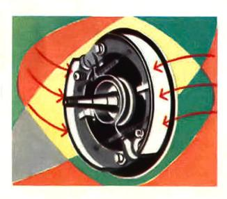
2 CYLINDER FRONT BRAKES apply braking pressure more evenly around the entire brake drum. The two shoes in each brake are forced evenly against the drum, Means more positive, controlled braking action.
