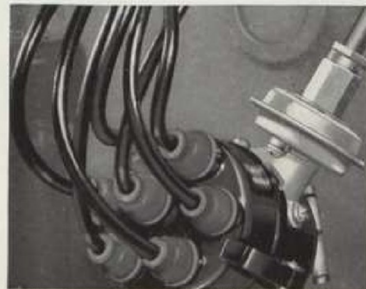
AUTOMATIC VACUUM SPARK CONTROL —In new Dodge, timing of the spark is automatically adjusted to the "pull" of the engine. This prevents knock. Saves gas. Improves performance.
