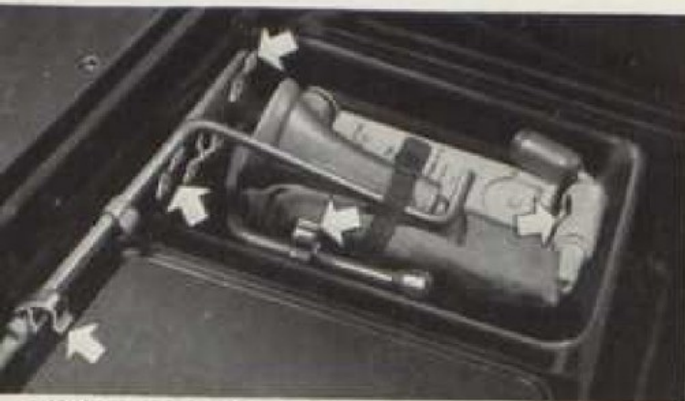
TOOL KIT CLIPS —Under Front Seat—Hold tools in place . . . always handy and ready for instant use. Tools carried under the rear seats of the Two-door Sedans.
