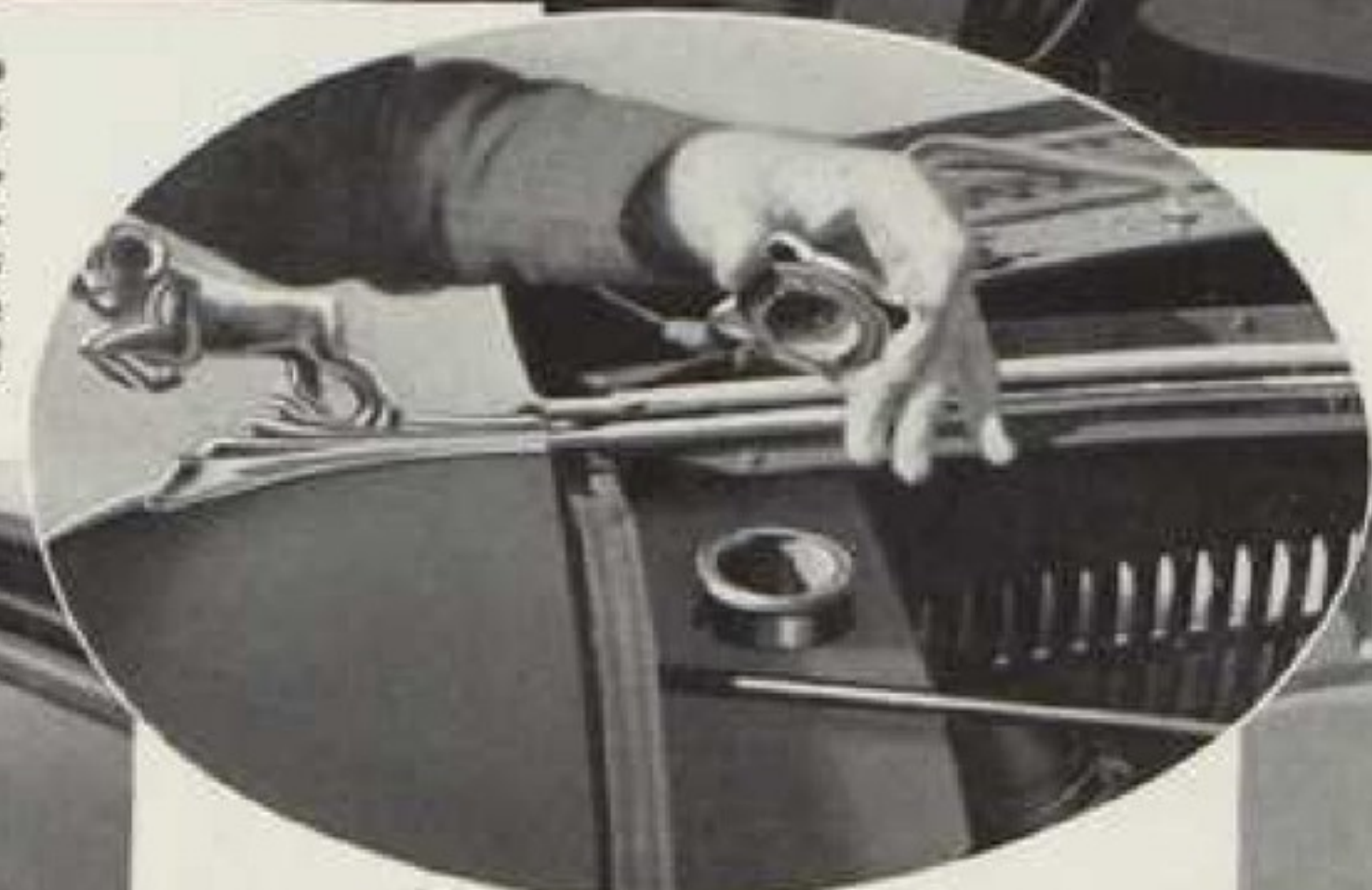
RADIATOR CAP UNDER HOOD —Another Dodge improvement. No more spilling anti-freeze solutions on the radiator shell or hood. And no more lost or stolen radiator ornaments. BIG PACKAGE SHELF IN COUPE —The shelf behind the seat in the Dodge Coupe for 1935 is 14 inches wide—plenty of room for parcels, brief cases, and for small luggage.
