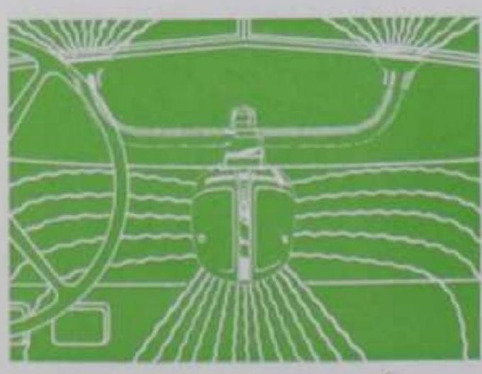
This new principle of mounting heaters in the center of the front compartment instead of at the side is used for both De Luxe and Standard models. It insures more even heat distribution and greater comfort for driver and passengers.
