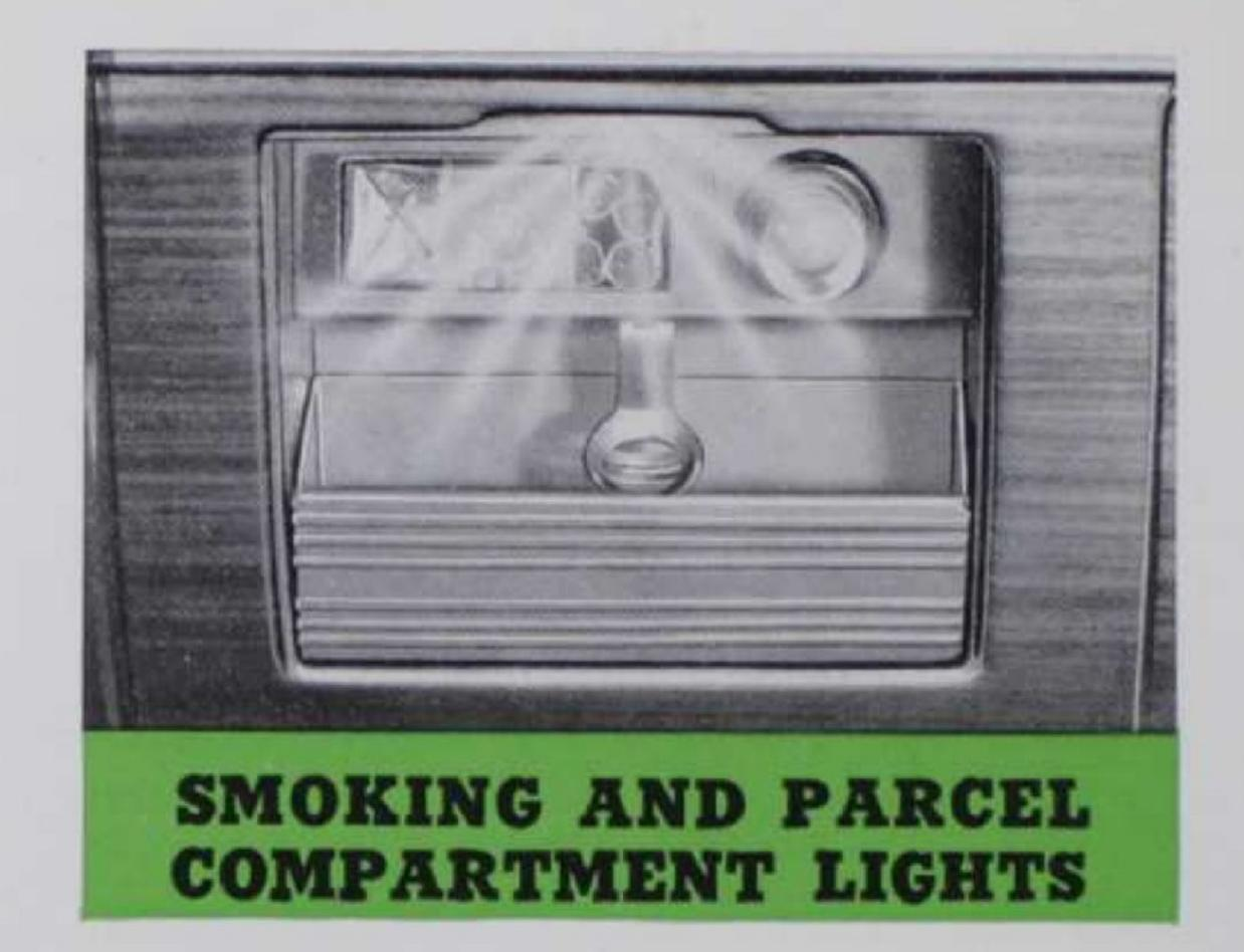
Two new convenience accessories that are appreciated by both driver and passengers. Lights brightly illuminate the interiors of the compartments. Provision has been made in all 1938 model Oldsmobiles for their installation. Lights for both compartments are sold as a combined installation.
