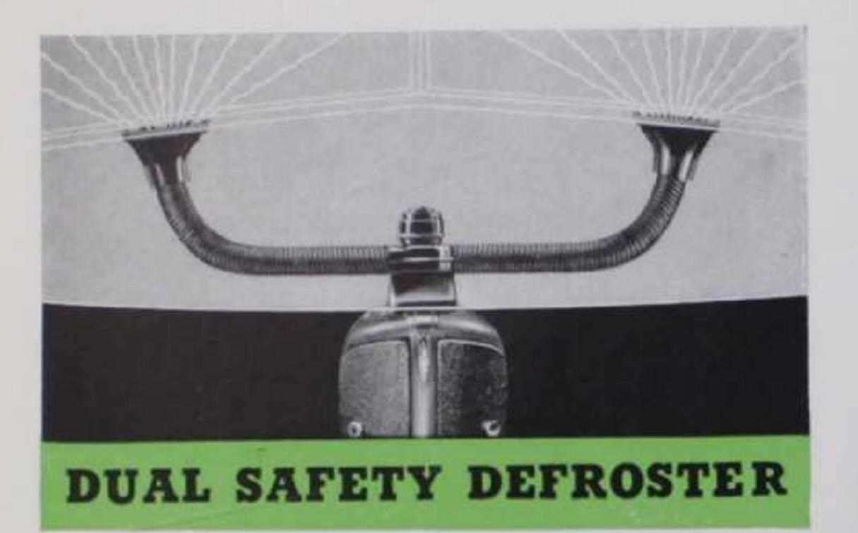
Designed for use with Oldsmobile's new 1938 Center Mounted Heaters. A steady flow of heat is directed against the windshield through two individually mounted, flexible tubes extending from heater to large vent openings at the top of the instrument panel. Controlled by a separate variable speed switch located in the Safety Instrument Unit. Clears frost, fog, snow and sleet from windshields very quickly and is a decided factor in safe driving.
