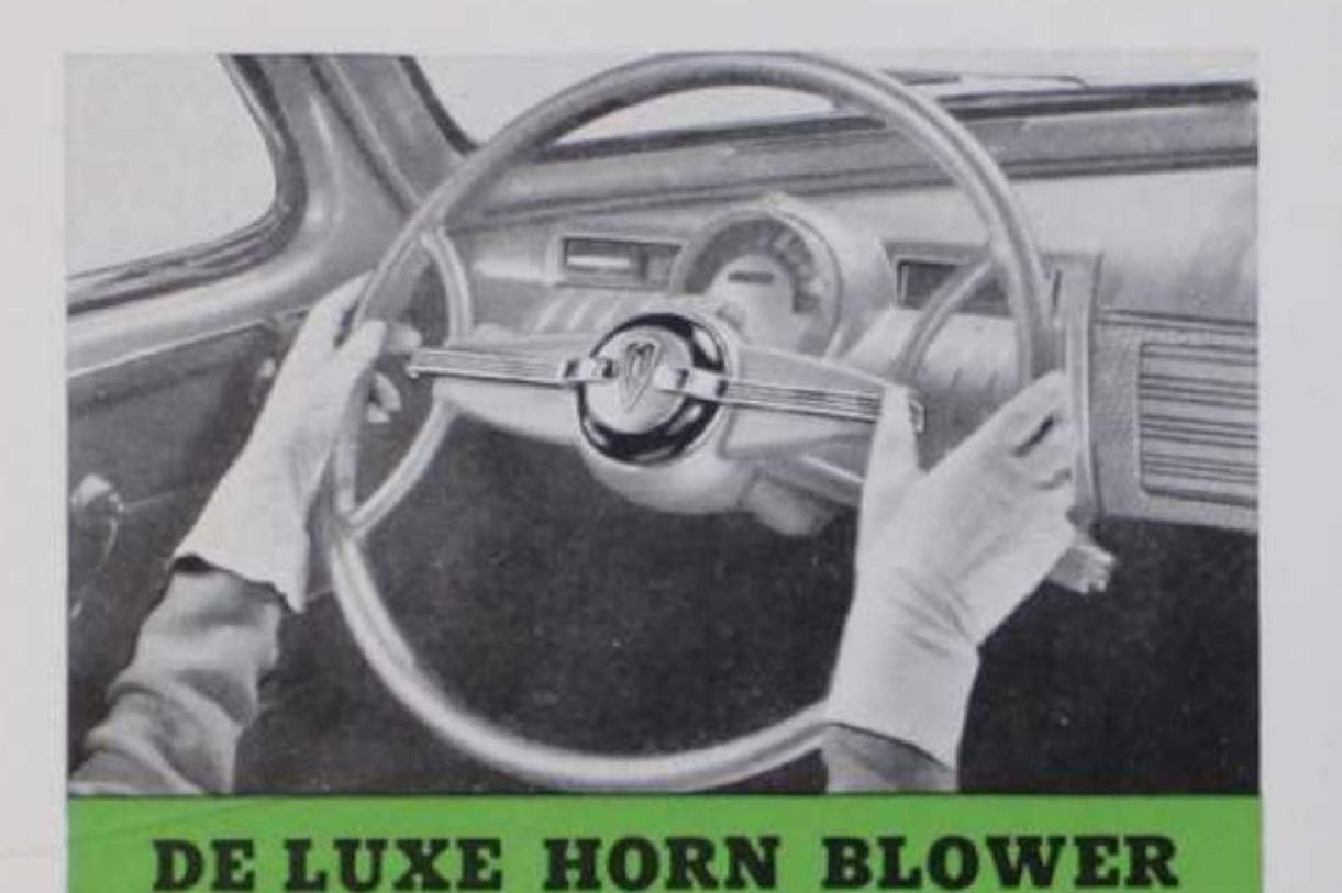
An exclusive Oldsmobile Safety Accessory that will prove convenient either when driving in heavy city traffic or at high speeds on the highway. Permits blowing the horn with either hand without removing hands from the rim of the wheel. Is attractively finished in chrome to harmonize with the instruments and interior fixtures of the car. Designed for installation only on the De Luxe Steering Wheel.
