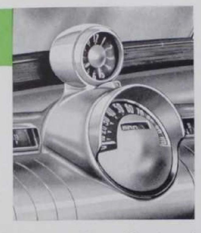
driver's vision and can be seen at a glance. Illuminated by a shielded light to make it easily readable at night.
