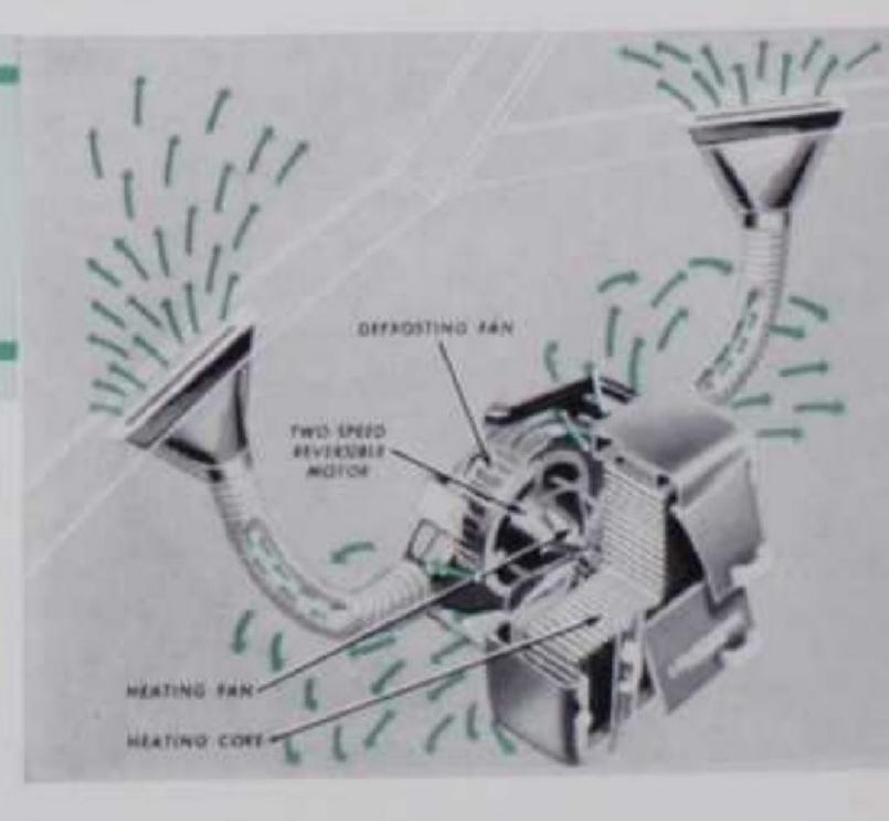
shield de-icing and directs sufficient heat from back of heater to warm car in moderately cold weather. "Indirect-Slow" position reduces volume for spring and fall driving. Switch in either position, with heater doors closed, directs car temperature air through defrosters.
