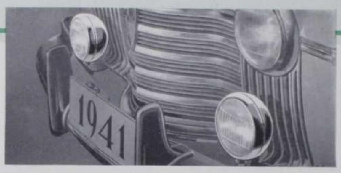
Greater visibility and safety when driving in fog, rain, dust or snow is provided by these specially designed auxiliary lights. They mount just below the headlamps and light up the area directly in front of the car, so giving greater light diffusion and reducing reflected glare. Operated by convenient instrument panel switch.
