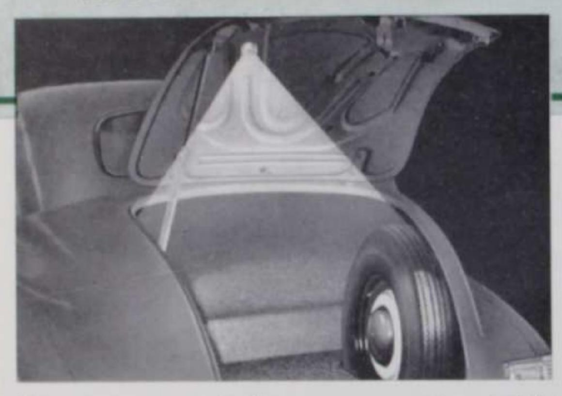
Placement or removal of luggage or spare tire at night is greatly facilitated with this convenient light that automatically illuminates the luggage compartment when lid is raised. Quickly attached to wiring already provided.
