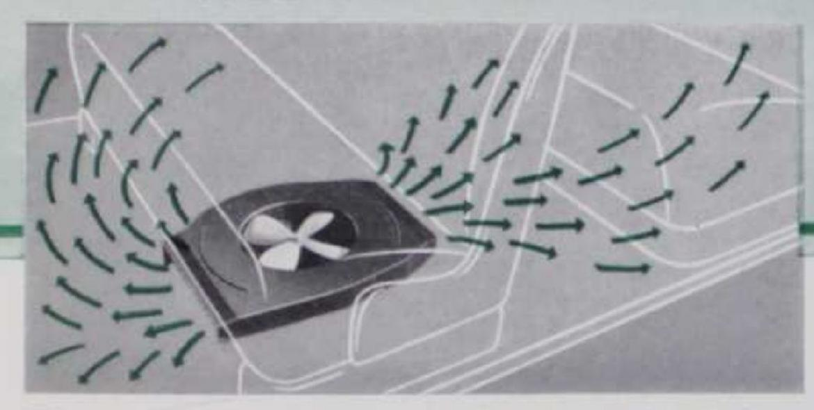
This modern heater operates efficiently and quietly to give all passengers in front and rear seats abundant warmth. Installed under the front seat at the left side, it concentrates a flow of heat on the floors eliminating drafts and permitting lower breathing level temperatures. Has illuminated variable-speed switch.
