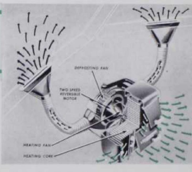
car temperature through defroster vents. After car is thoroughly warmed, switch turned to "Direct-Slow" position maintains warmth in all but most severe weather. In either switch position, optional windshield defrosting with air of car temperature is possible.
