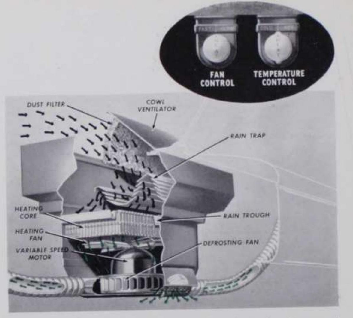
Fresh air in large volume enters through the cowl ventilator, where it is freed from dust, dirt, rain and snow by a special filter and rain trap. Then it is warmed to the desired temperature by the large heating core and forced by pressure of the car's movement into and throughout the car. Pressure forces out used air at all ordinary driving speeds and keeps outside air from seeping in.
