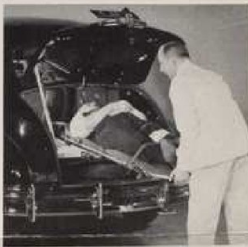
ROLLING STRETCHER INTO CAR. Stretcher is set on tracks, then rolled into place. Winged nut locks stretcher in place, prevents it rolling backwards. Trunk door is lowered and Nash ambulance is ready to proceed.
