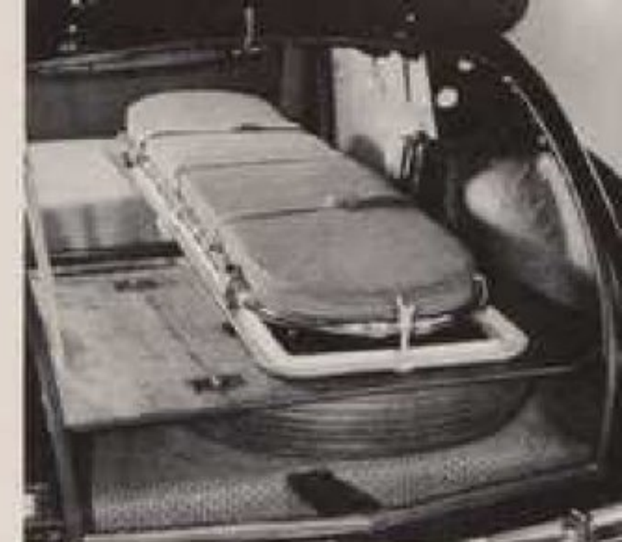
ROLLER STRETCHER in position on stretcher track. Stretcher is anchored into place by means of a bracket and winged nut. Special straps on stretcher hold patient securely while car is in motion.
