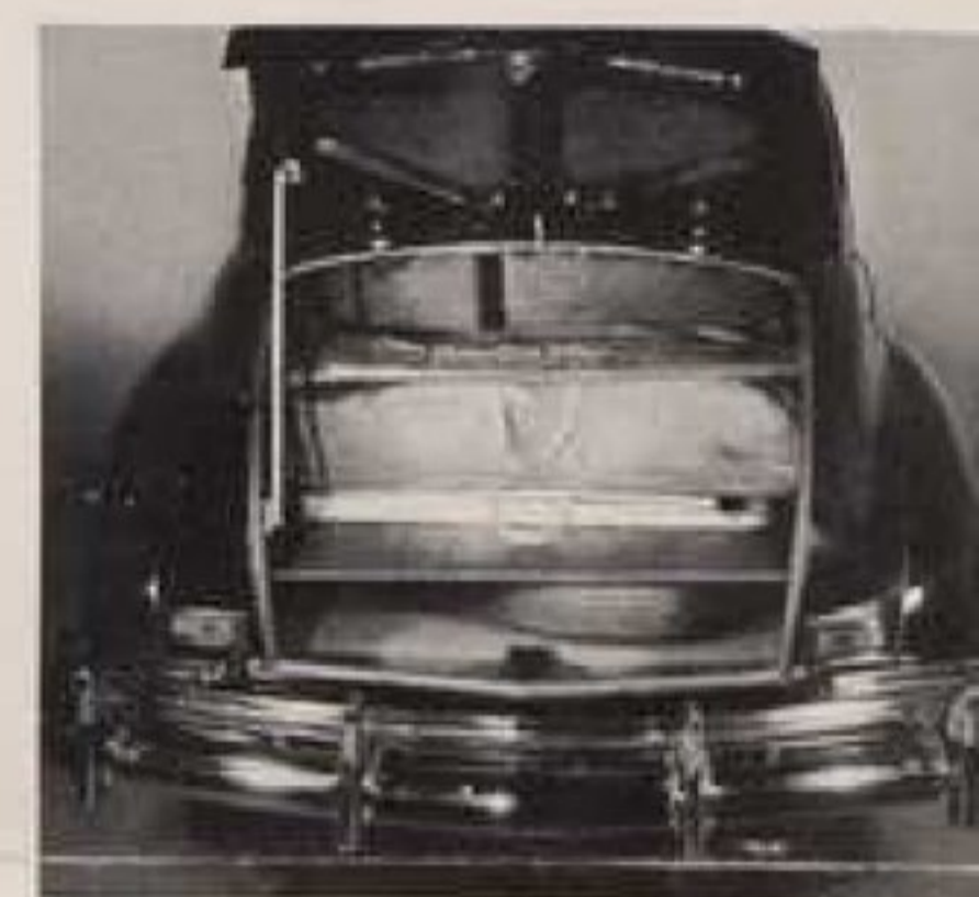
WHEN NOT IN USE all this ambulance equipment conveniently packs away neatly in trunk compartment, leaving rest of car free for normal use—a dual-purpose car for emergencies—makes up in one minute flat!
