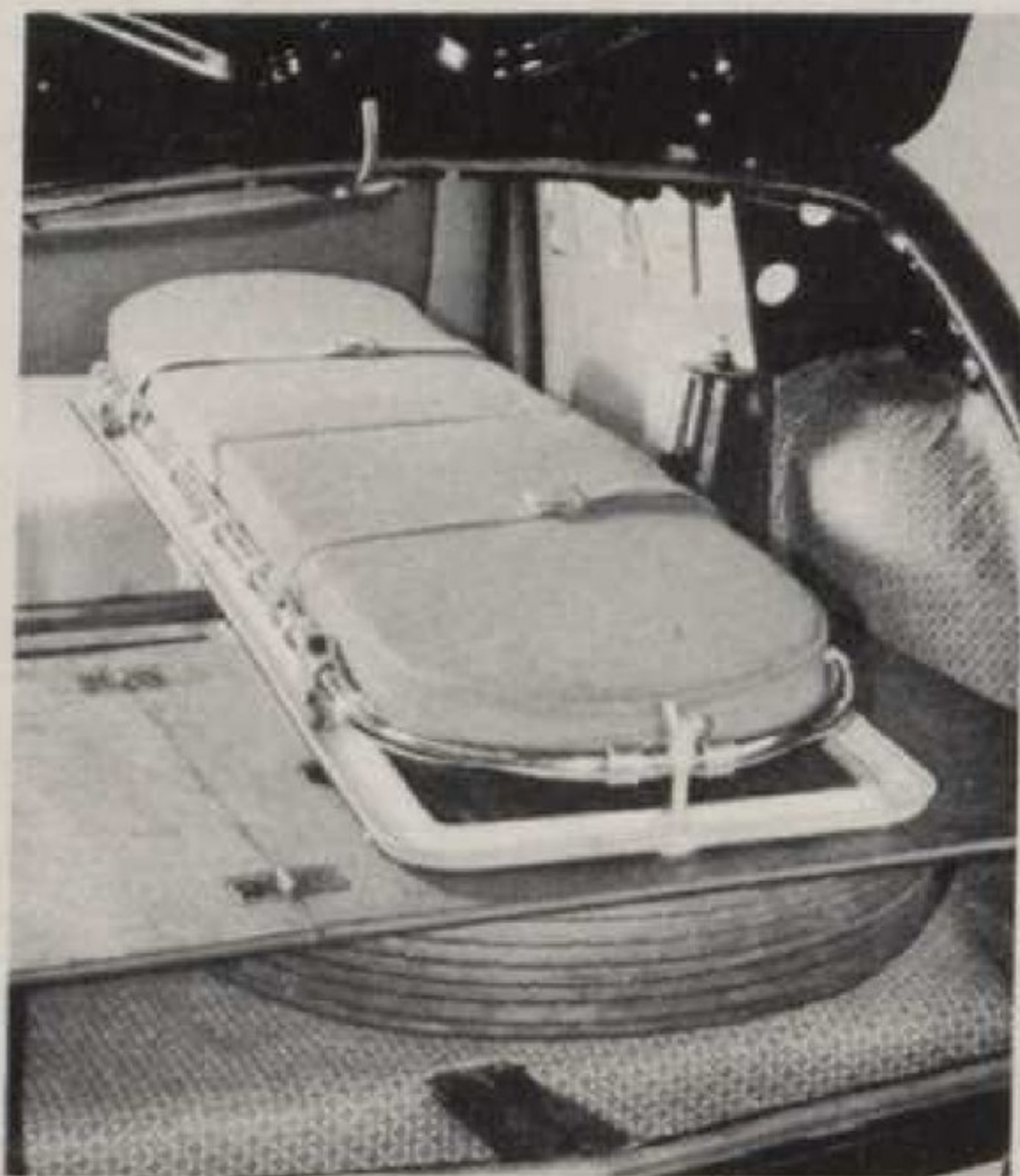
THE ILLUSTRATION ABOVE shows the installation of the emergency ambulance equipment. The appearance of the car is not altered in any way and it can be instantly converted into an ambulance.
