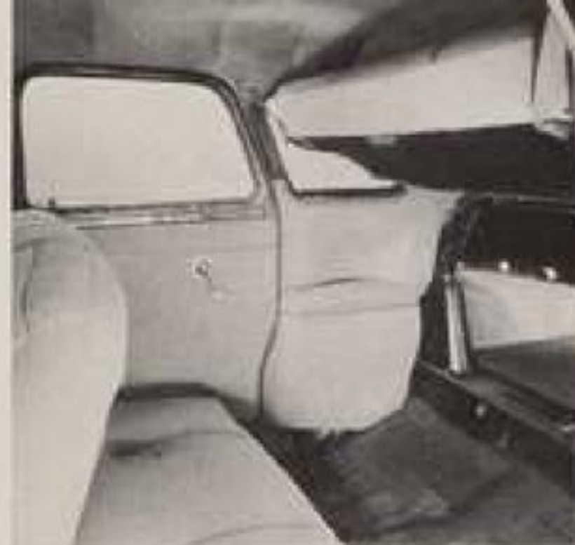
IN EMERGENCIES the rear seat cushion is pulled forward on compartment floor, and the rear seat back is raised, providing room for the special ambulance equipment. Taken only one minute, one man to do this.
