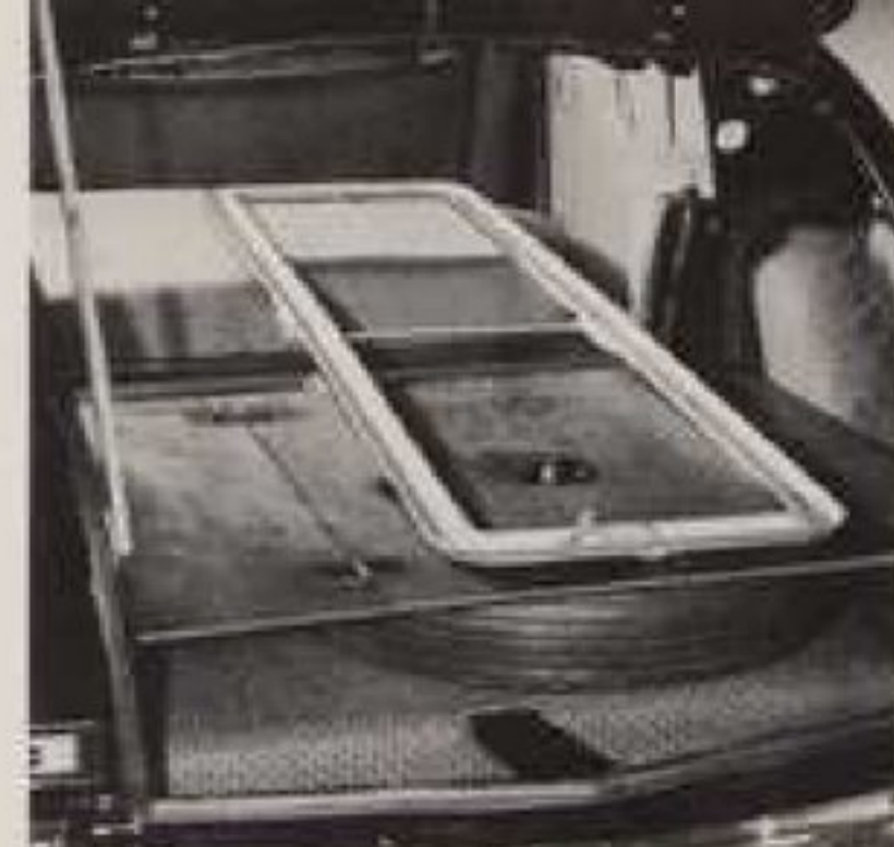
STRETCHER TRACK is shown in place, one end resting on rear seat cushion and other end supported by special plywood shell over spare tire in trunk compartment. Shell is secured in place by a single winged nut.
