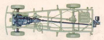
CHASSIS of the sensational 4-wheel-drive 'Jeep' Truck, showing two live axles that give tractive effort on all wheels. Note transfer case, back of transmission, which permits selection of 2-wheel drive, or 4-wheel drive with 6 speeds forward, 2 reverse. Optional power take-off is operated by shaft from rear of transfer case.
