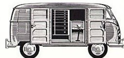
A repairman can build-in binned storage space for tools, parts.
