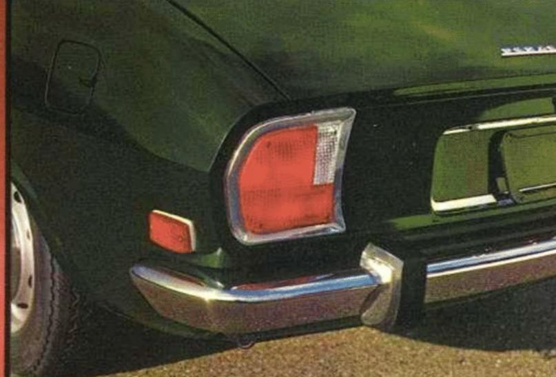
At the rear: fully separate systems for tail lights, turn signals and emergency flashers, brake lights, back up lights. Rubber covered bumper guards. Spare tire on rack beneath trunk is accessible from exterior (no need to unload trunk).
