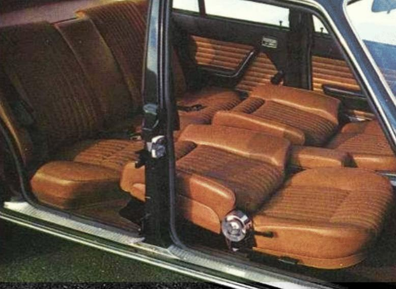
When we say fully reclined seats...we mean flat out! Retractable headrests make this possible. Front seats slide back and forth on curved rails (ball bearings, spring return), automatically adjusting to the height of all size drivers.
