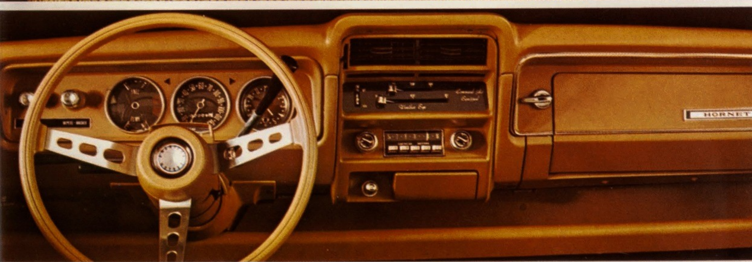
Left: Hornet Instrument Panel. New 3-Spoke 15" Sports Steering Wheel, optional (standard in Hornet "X"). Two new Radios, optional: AM Push-Button (same quality as Javelin's), AM/FM Push-Button (monaural). Lockable Glove Box, standard. Package tray—Full width of instrument panel, standard.
