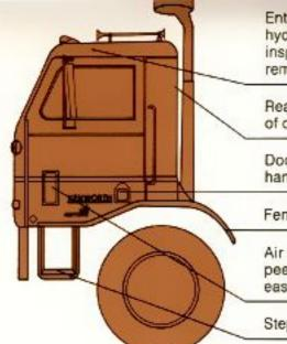
Entire cab assembly tilts forward hydraulically for maximum ease of engine inspection and repair. A dash light reminds driver when cab is not securely latched.
