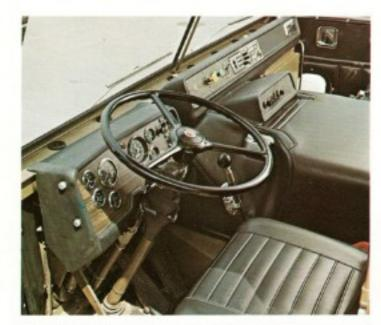
The dashboard is molded Cycolac® that's sturdy and yet attractive with a wood-grained finish insert. Black dial, side-illuminated instruments are easy to read and meet the latest RCCC recommendations—being grouped according to importance and frequency of use.
