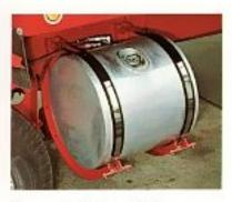
Kenworth builds all its own aluminum fuel tanks. The 50-gallon size is standard, and optional sizes range up to 105-gallons. In all tanks, the fuel line connection and gauge-sending unit is recessed for greater protection. The HUSTLER has aluminum brackets rather than just straps for fuel-tank mounting. This superior design, along with nylon-lined straps, insures proper seating and support for the tanks.
