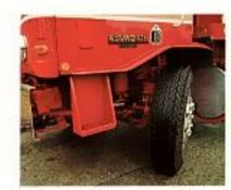
The HUSTLER's outstanding urban maneuverability is the result of Kenworth's steering geometry. A turning angle of up to 40° is achieved by positioning the steering gear forward of the front axle. This makes the HUSTLER easy to handle in a variety of applications.
