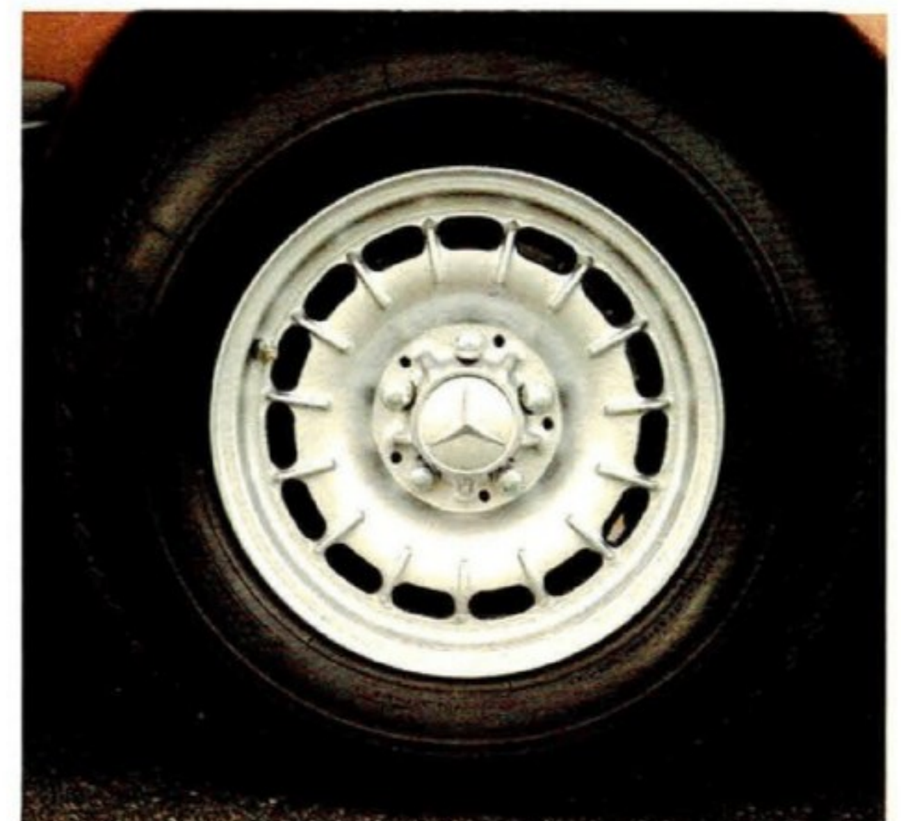
Light alloy wheels provide additional cooling air to the four disc brakes.
