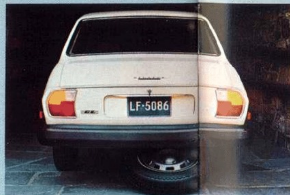
You never have to unload to get to the spare. It's mounted underneath the car.
