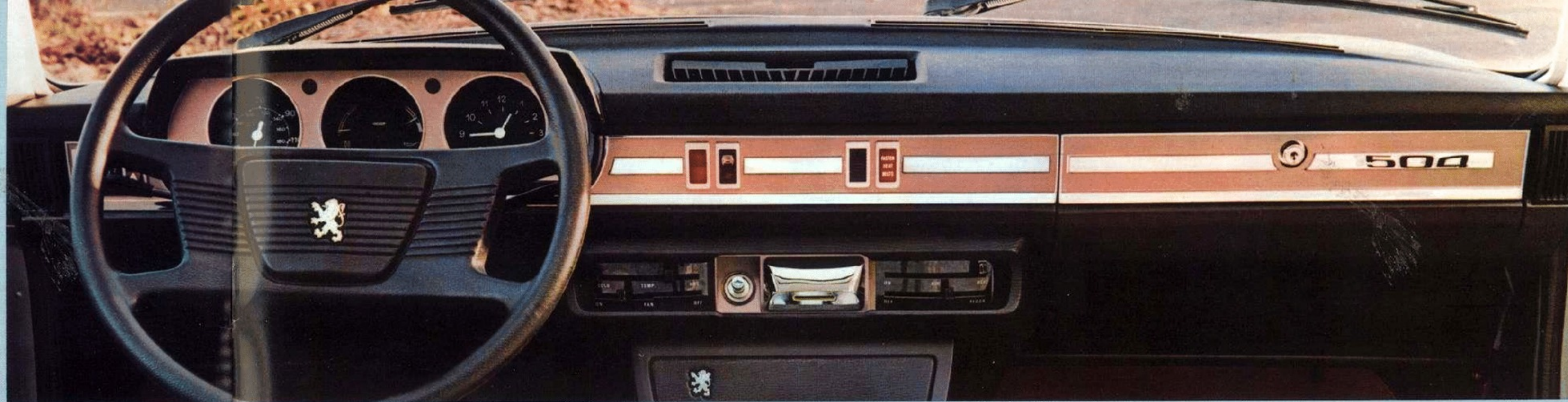
Padded steering wheel connects you to the front wheels in the most direct way: via rack and pinion steering.
