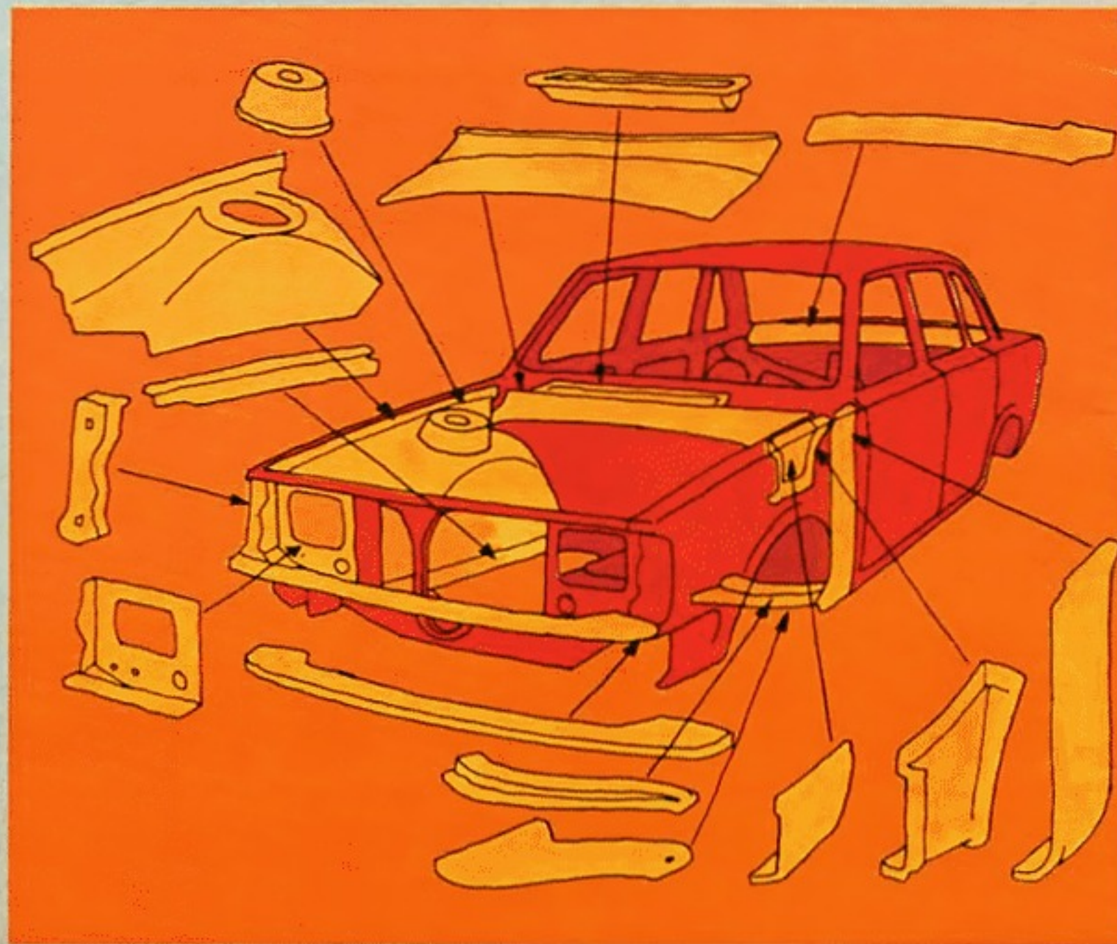
The use of hot-dipped galvanized sheet steel for areas most susceptible to rusting, including those to which safety related components are mounted, are shown in this drawing. Other examples of corrosion resistant materials are the aluminum alloy and stainless steel trim.
