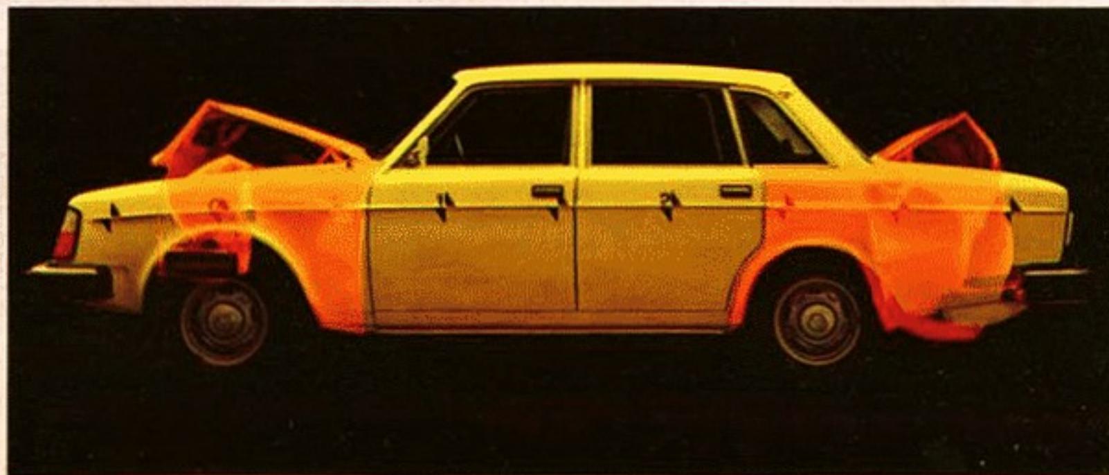
Rigid members of the body form a protective cage around passengers. In addition to pillars and side-guard bars, the floor pan is reinforced by a large traverse box section. Special patterns stamped into the panels of the built-in "crumple zones" allow major impacts to be absorbed at controlled rates.
