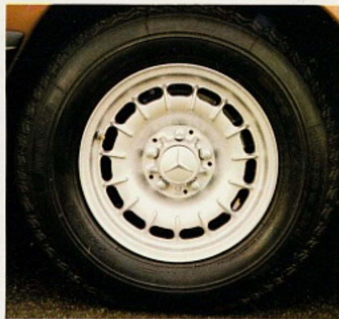
Light alloy wheels provide additional cooling air to the four disc brakes.
