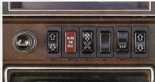
CENTRE CONSOLE , with cigarette lighter and finger tip controls for electrically operated windows.
