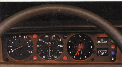
INSTRUMENT PANEL , with speedometer, tachometer and electric clock set behind anti-reflective glass. Warning lights, including those for brake condition, lights and indicators are grouped around the circular dials, designed to be read in a single, swift glance.
