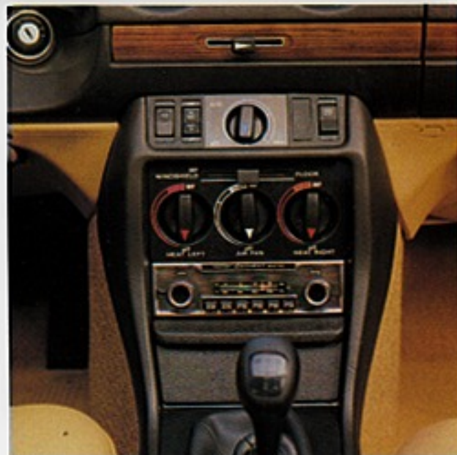
Heating system lets you select separate temperatures for right and left sides of car. Radio and air conditioner shown optional at extra cost.
