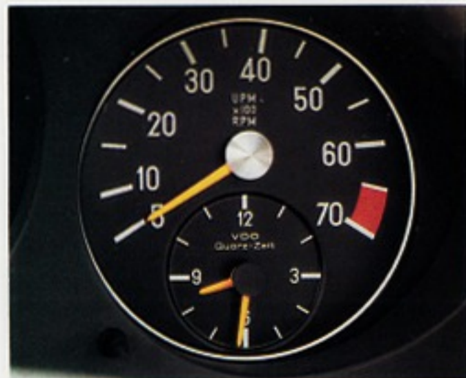
Complete instrumentation includes a tachometer and quartz chronometer.
