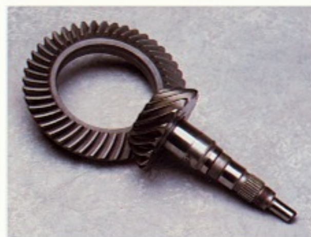
Changes in final drive ratios are an uncomplicated way to increase acceleration.
