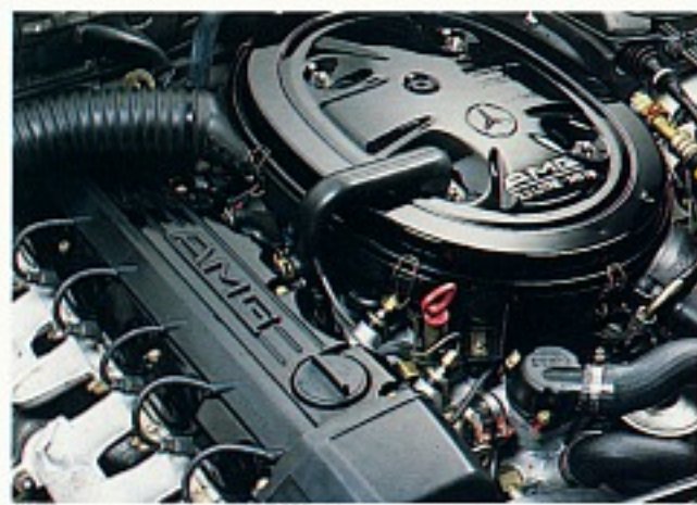
The 3.2-liter engine conversion increases power by 38 percent over the standard 3.0-liter motor.
