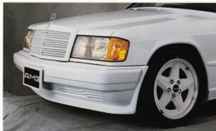
190E alloy wheel choices include 6.5 × 16 for all models up to 1986 and a 7.5 × 16 version for 1987 models.
