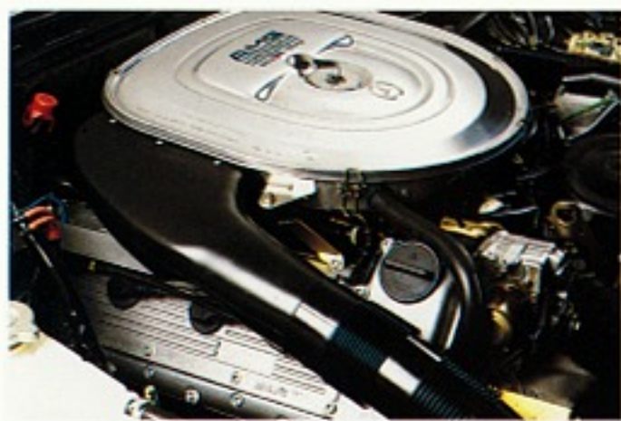
Power choices range up to a Herculean 375 hp, 6.0-liter 4-cam replacement of the standard 5.6-liter engine.
