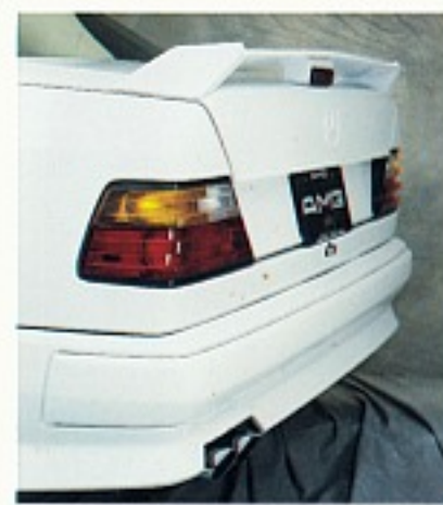
The 300E spoiler has a brake light for maximum safety.
