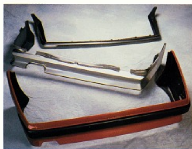
Bottom left to right; rear skirts, front air dams and side skirts for S-Class and 300E models.
