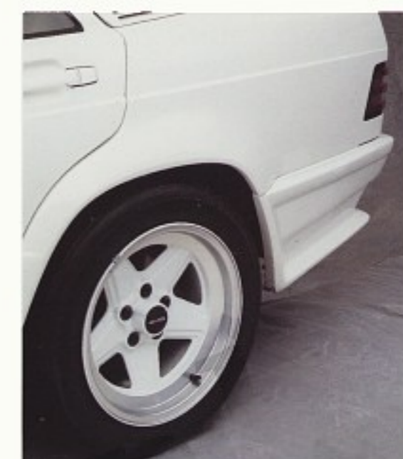
The 190E Wide Body front and rear fenders yield more room to accommodate the widest possible wheel sizes of 8.0 x 16 or 8.0 x 17.
