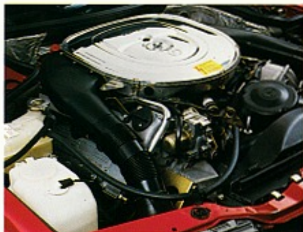
Standard motive power is the 5.6-liter 4-cam engine. Optional is a 375 hp 6.0-liter version.
