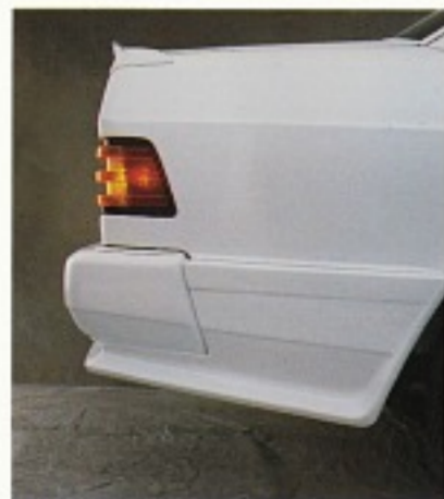
This spoiler succeeds in a 40 percent reduction of rear end lift.
