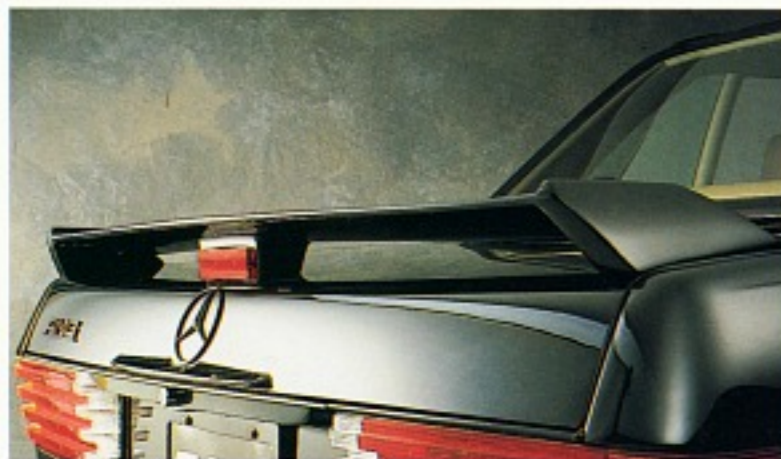
The rear wing spoiler with high-mounted brake light updates older models to contemporary safety standards.
