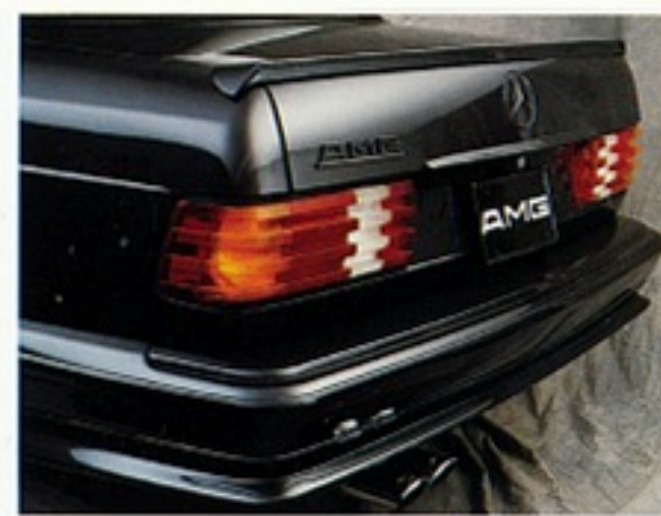
This rear spoiler strengthens road grip through a reduction in rear end lift.
