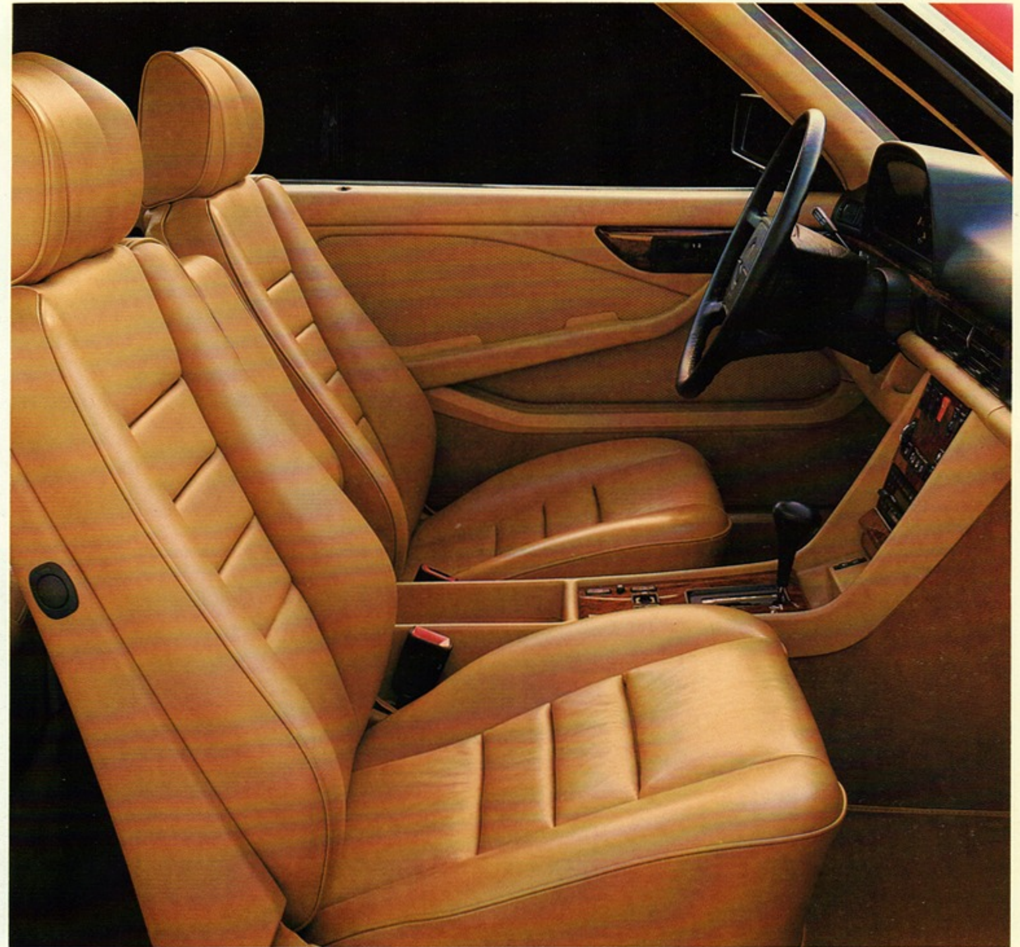
Below: Individual bucket-type seats are fitted in the rear as well. Note plump folding center armrest. The front seatbacks are normally locked in place with the engine running; to facilitate entry and exit for those in the rear, the seatbacks automatically unlock whenever either door is opened. The door itself is very wide to enhance access to the rear seat area.
