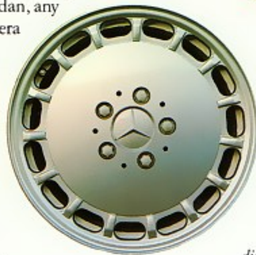
Slotted, disc-smooth forged light-alloy wheels, as shown at left, are standard on all S-Class cars. Their advantages are threefold: reducing unsprung weight, venting heat generated in hard use away from the brake discs, and shaped to help reduce aerodynamic drag.
