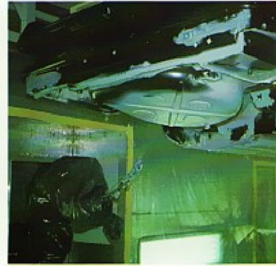
Far left, hand workmanship continues to play an important role in the construction process. Here, a skilled metal worker smooths a raw metal body prior to painting. Left, robot sprays the underside of a car with thick PVC undercoating. Over 30 pounds of this protective material is applied to every Mercedes-Benz.
