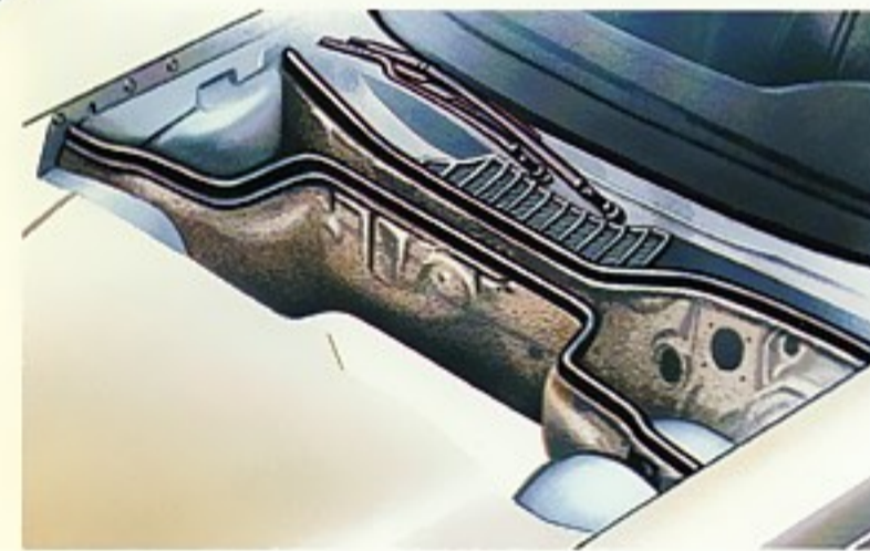
All S-Class sedans and the 560 SEC Coupe are fortified against engine noise by an ingenious second firewall, forward of the main firewall. The space between them harbors heat-sensitive aggregates such as the battery and certain electricals.
