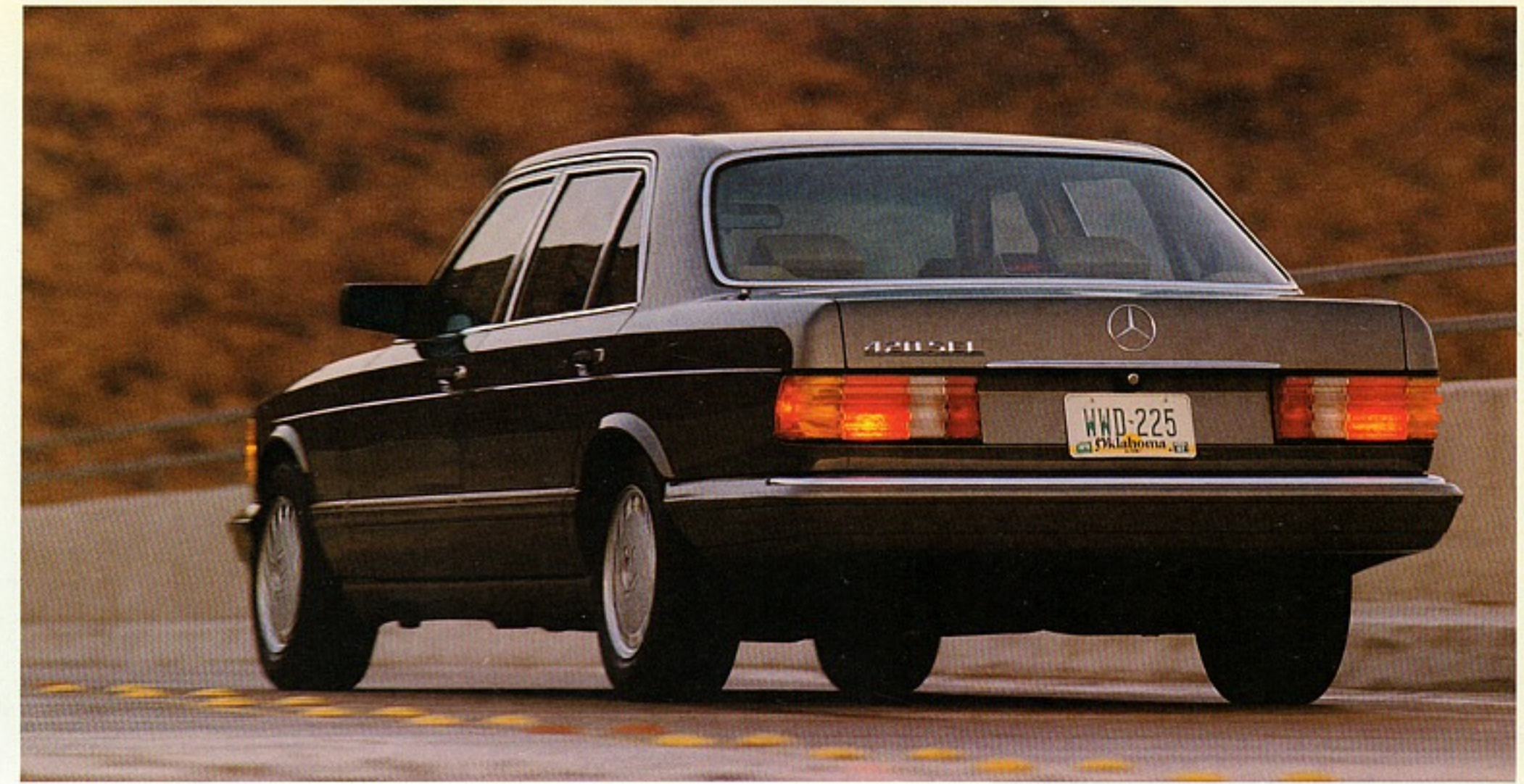
Right: Mercedes-Benz body design is governed by the search for functional efficiency; one result is a striking absence of excess brightwork and decoration; another is a very low 0.37 coefficient of aerodynamic drag. The photo on the page opposite shows the wiper fitted to each halogen headlamp; individual headlamp washers are a further aid to driving visibility in foul weather conditions.
