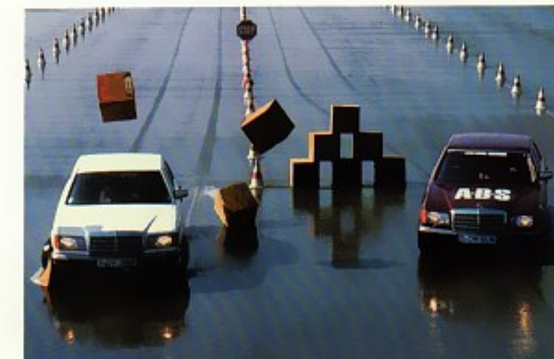
This test car will avoid the barrier. The ability an ABS-equipped car gives its driver to brake and steer his way out of trouble, in situations that might otherwise pose severe hazards, ranks as one of the major advances in driving control in recent years.
