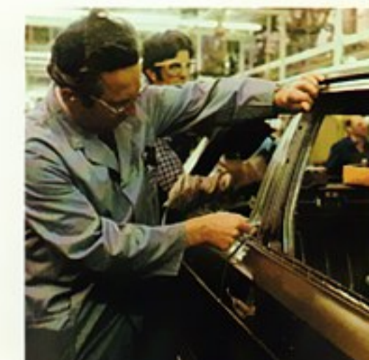
Near the final stage of the assembly process, an inspector using a special instrument checks the tolerance of door fittings. At Mercedes-Benz, automation and robotics will always be subject to the ultimate arbiter of the trained eye, the experienced hand, and the judgment of acceptable quality that only the human mind can make.
