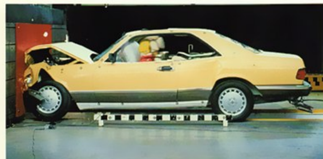
Computers and simulators have obviated some of the need for real-world testing procedures connected to the development of Mercedes-Benz automobiles, but the engineers have found no satisfactory substitute for the carefully monitored crash test, using samples from the production line. Left: A new 560 SEC Coupe is sacrificed in a duplication of a frontal impact at highway speed.
