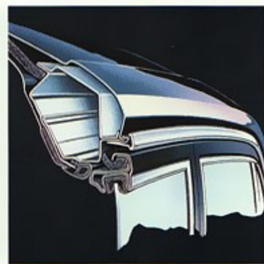
Long famed for hand-workmanship, Mercedes-Benz was also one of the first practitioners of advanced robotics in the automotive industry. In welding operations like that at left, for example, robots are tireless. And inhumanly precise. Right, detail of roof rail design combining strength and lightness.
