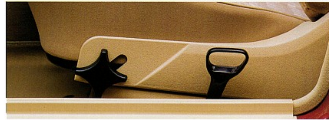
New trim around the base of the seats, so they blend into the floor carpeting.
