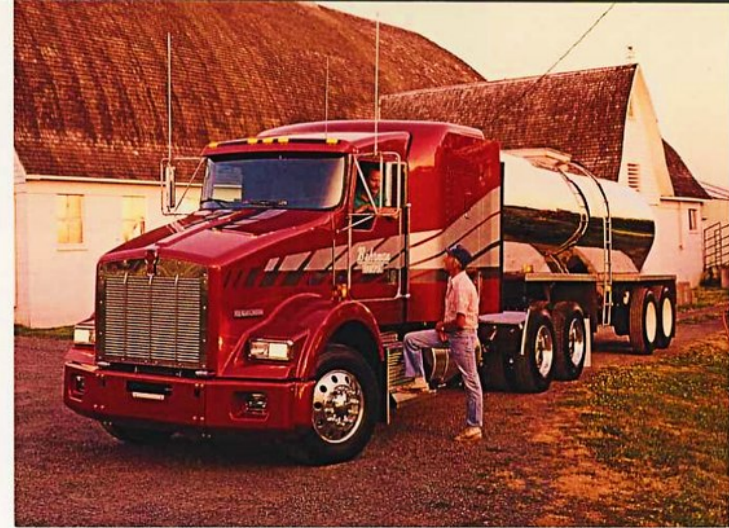
Ideal for tanker applications, the AeroCab FlatTop offers a low profile roofline which still provides six feet of stand-up sleeper headroom
